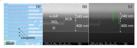
Fig. 6. (a) Array of printed III-V coupons on a silicon photonic target substrate (before photoresist encapsulation removal). (b) Cross section image at end of the coupon; (c) Cross section image in the middle of the coupon.
