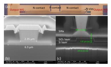
Fig. 8. (a) Top-view microscope image of a transfer-printed DFB laser, (b) FIB cross section image in the middle of the DFB laser, (c) FIB cross section image near the III-V/Si taper tip, showing a misalignment of less than 250 nm.
