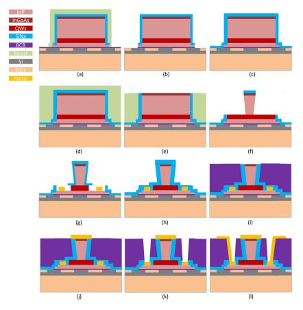
Fig. 7. Process flow for the definition of the III-V mesa structure in the transfer-printed coupon. (a) Transfer printed III-V coupon onto Si PIC, (b) Resist removal, (c) SiN deposition, (d) Resist planarization, (e) Etching back to expose the p-InGaAs layer, (f) Laser mesa and taper definition, (g) QW patterning and n-contact metal deposition, (h) SiN passivation, (i) DVS-BCB planarization, (j) p-contact metal deposition, (k) n-via opening, (l) Final Ti/Au metallization.
