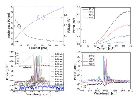
Fig. 9. Performance of the fabricated DFB laser. (a) V-I curve and differential resistance, (b) P-I curve at different temperatures, (c) Superposition of the output spectra at different bias currents, the inset shows the laser wavelength evolution as a function of current (d) Wavelength shift as a function of the stage temperature.
