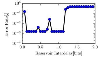
Figure 6. Error rate vs reservoir interdelay for the single-mode reservoir for the 3 bit header recognition task.
