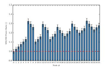
**Figure 10.** Comparison of single-mode and multimode 36 node reservoir average power per node for input to node 0.
