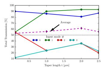
**Figure 4.** Total transmission (summed over all output modes) in the Y-junction combiner for different taper lengths. Results are shown for input to the upper arm of the junction consisting of the fundamental (0), 1<sup>st</sup>, 2<sup>nd</sup> and 3<sup>rd</sup> order modes as well as the average transmission across all input modes. The baseline transmission of 50%, for the adiabatic single-mode Y-junction, is also indicated.
