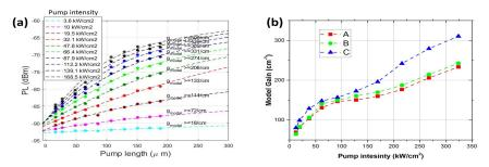
Fig. 2. (a) Experimental data of measured ASE as function of the pump length and for different pump intensities. (b) Fitted modal gain  $g_m$  as a function of pump intensity for sample A, B and C.
