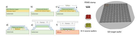
Figure 1 Transfer printing integration approach.
