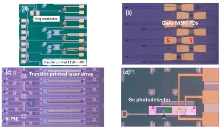
**Figure 2** Demonstrations of the transfer printing technique for photonic integrated circuits: a) integration of O-band photodiodes on an iSIPP25G full platform silicon photonic IC; b) 850 nm GaAs MSM photodetectors on a SiN waveguide circuit; c) C-band etched facet laser integration on a passive Si waveguide circuit; d) a silicon-waveguide coupled Ge high-speed photodiode integrated on a passive silicon waveguide circuit.
