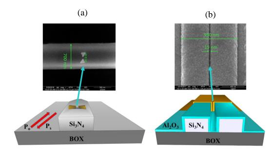
Fig 1. The schematic of the  $Si_3N_4$  integrated SERS sensors. a) The bowties antenna integrated a monomode  $Si_3N_4$  strip waveguide. b) The plasmonic waveguide interfaced with a monomode AlO clad  $Si_3N_4$  slot waveguide. The inset shows the SEM image of the fabricated sensor.
