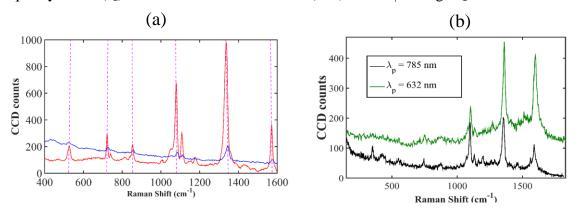
Fig 1. a) The Raman spectra of 4-Nitrophenol measured from a bowtie antenna (blue) and a metal slot waveguide (red) integrated with SiN waveguide. The pink dotted lines represents the Raman modes of NTP. b) The Raman spectra measured from a metal slot waveguide at 785 nm (black) and 632 nm (green) excitation wavelengths.
