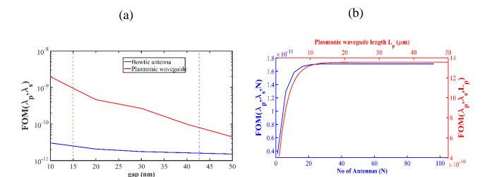
Fig 2. The calculated figure of merit (FOM) for a bowtie antenna (blue) and a plasmonic waveguide (red). a) The FOM as a function of plasmonic gap and b) interaction length (No of antennas for an antenna array and waveguide length for a plasmonic waveguide).
