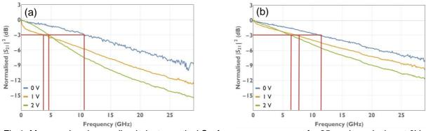
Fig 1. Measured and normalised electro-optical S<sub>21</sub> frequency response of a 25 µm long device at 0V, 1V and 2V DC bias voltages, for (a) standard doped and (b) highly doped Si waveguide.
