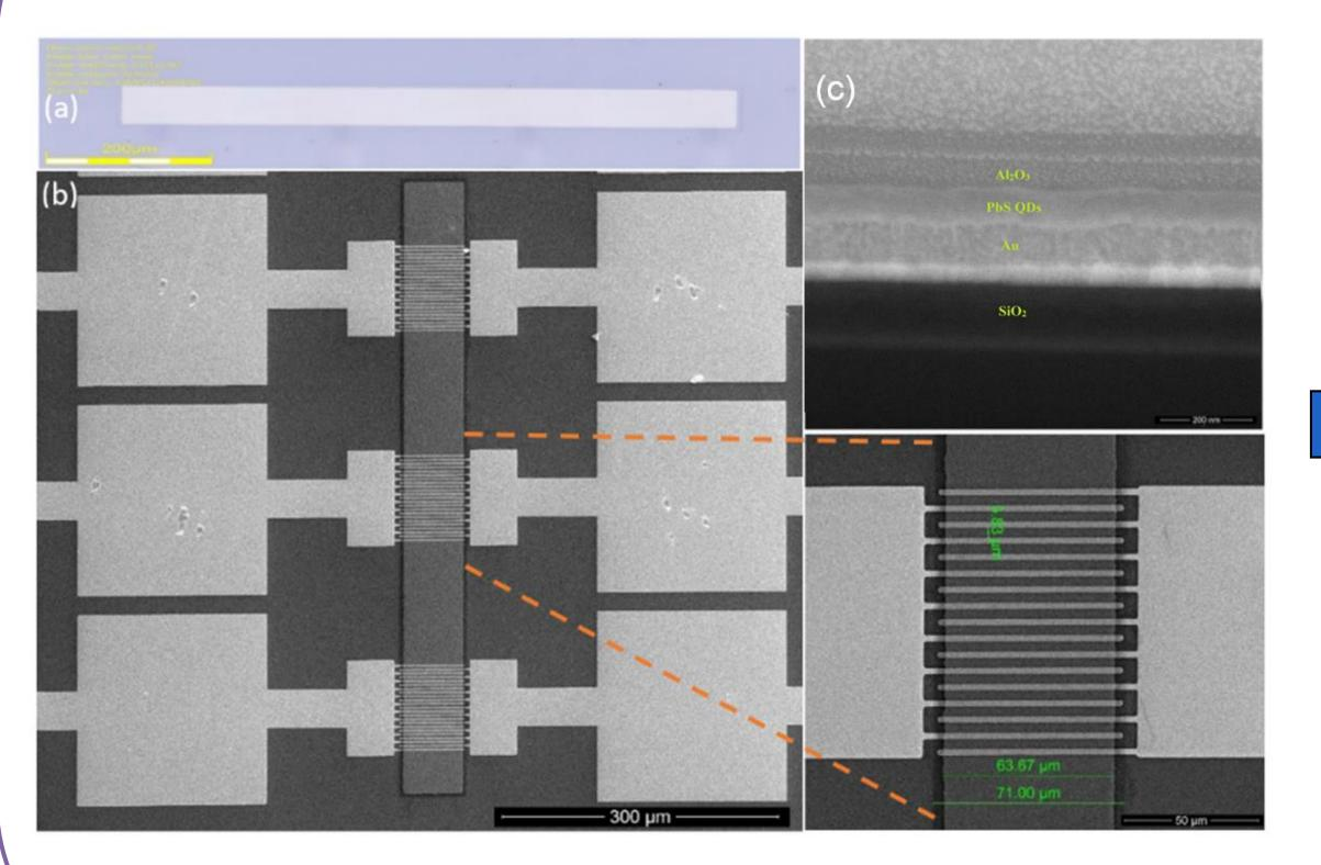
Fig.3 (a) optical image of the source substrate after pattern pick-up, (b) Printed Al2O3/PbS QD photoconductor, and (c) cross section.
