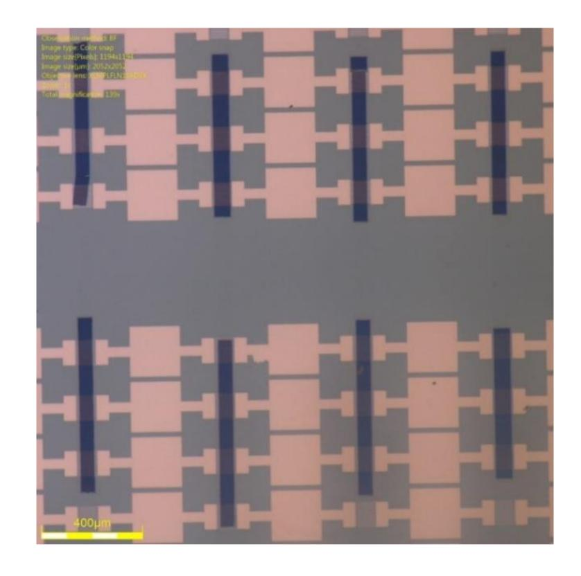
Fig.2 Integrated Arrays of printed Al<sub>2</sub>O<sub>3</sub>@PbS<sub>2.1µm</sub> QD photoconductors
