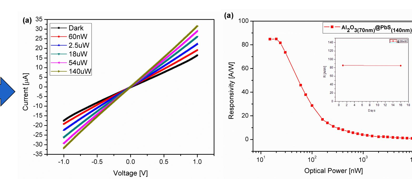
Fig.4 (a) IV characteristics in dark and under surface illumination at 2.1 μm, and (b) corresponding responsivity and (inset) life-time stability
