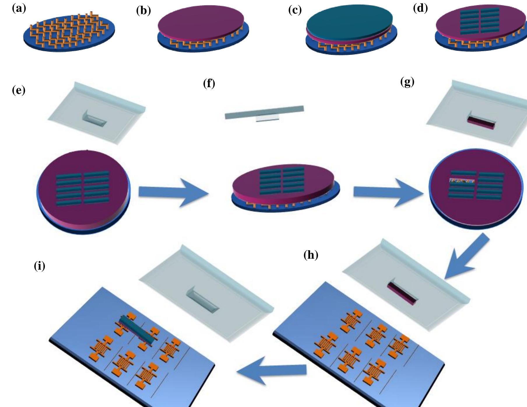
Fig.1 (a-d) **Source substrate preparation**, including ODTS-Si preparation, QDs spin coating and ALD-Al<sub>2</sub>O<sub>3</sub> encapsulation. (e-i) **Pick-and-Print** of Al<sub>2</sub>O<sub>3</sub>/PbS patches on interdigitated electrodes on an oxidized Si wafer
