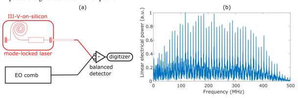
Figure 2: (a) An overview of the measurement set-up use to generate the dual-comb set-up. (b) The spectrum generated by taking the Fourier-transform of 1 us slice of the dual-comb interferogram.
