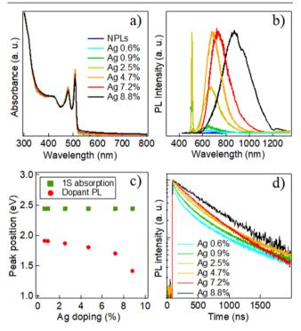
**Figure 2.** (a) UV—vis absorbance spectra of CdSe:Ag NPLs at increasing Ag concentration. (b) Corresponding steady-state PL spectra ( $\lambda_{\rm ex} = 400$  nm, same color labels as the absorbance spectra). (c) Plot of the PL peak position against Ag concentration, highlighting the red shift of the dopant emission (red dots), whereas the BE absorption remains fixed (green squares). (d) PL decay traces of the dopant emission for different doping concentrations.
