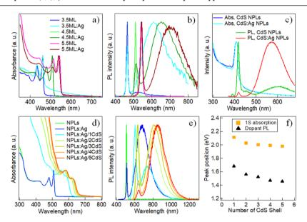
Figure 5. (a) Absorption and (b) PL spectra of CdSe and CdSe:Ag NPLs with thicknesses of 3.5, 4.5, and 5.5 MLs. (c) Absorption and PL spectra of CdS and CdS:Ag NPLs. (d) Absorption and (e) PL spectra of 4.5 ML CdSe:Ag NPLs and the corresponding CdSe:Ag/CdS core—shell NPLs with different number of CdS MLs. (f) Change of the BE absorption and dopant PL peak positions with the number of CdS shell layers.
