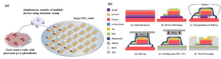
Fig. 1. Schematics of (a) micro- transfer printing on wafer-level scale and (b) the device fabrication and µTP process on a component level.
