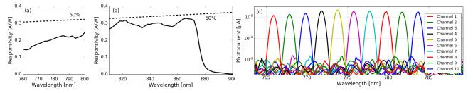
Fig. 3. The measured responsivity of the waveguide-coupled PD (a) from 760 nm to (b) 900 nm. (c) Shows the measured photocurrent of the AWG output PDs.
