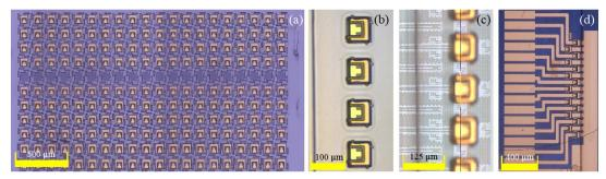
Fig. 2. Microscope images of (a) the source substrate with pre-processed PDs, (b) multi-PD pick-up on the PDMS stamp, (c) visual alignment and printing on top of the AWG channel output GCs and (d) the final interconnected system after post-processing (planarization, VIA access and metallization).
