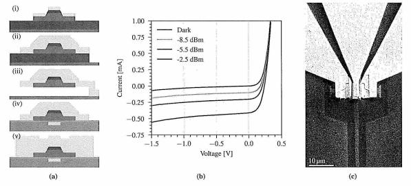
Fig. 1 (a) Fabrication steps, (b) IV-curves for different incident on-chip powers, and (c) SEM-image of a  $2 \,\mu m \times 10 \,\mu m$  waveguide-coupled UTC PD.
