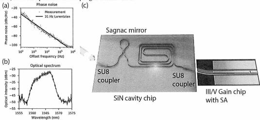
Fig. 1. (a): The measured phase noise of the 2.18 GHz fundamental beat note and the 31 Hz wide Lorentzian fit. (b): Optical spectrum of the laser. (c): artistic view of the mode locked laser, with the lensed fiber outcoupling on the left
