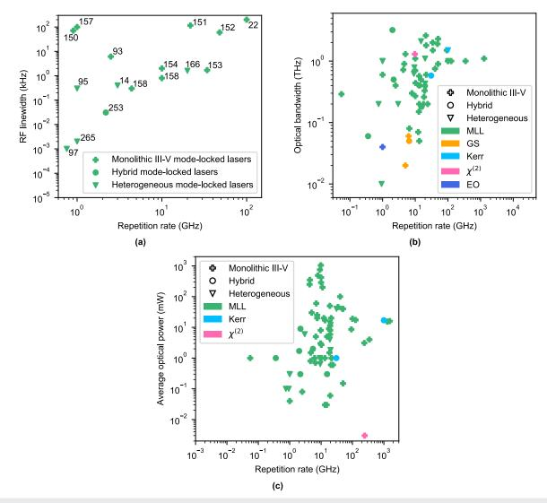
FIG. 8. (a) RF linewidth vs repetition rate for on-chip passively mode-locked lasers emitting at a wavelength of 1.6  $\mu$ m. The references corresponding to the data points are indicated in the figure. (b) Optical bandwidth vs repetition rate for the on-chip optical comb sources listed in Tables III–VI. (c) Average optical output power vs repetition rate for the on-chip optical comb sources listed in Tables III–VI.
