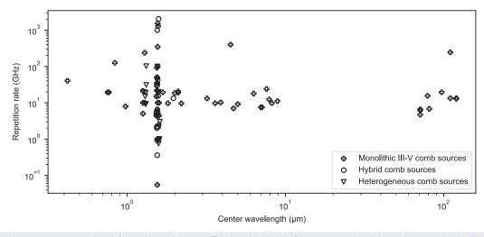
FIG. 7. Repetition rate vs center wavelength for on-chip comb sources. The data plotted in this figure correspond to all the comb sources listed in Table III-Table VI.
