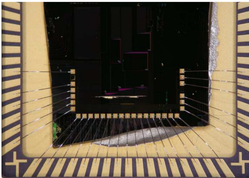
Figure 2 - 18. Photograph for the complete set of 30 III-V photodetectors bonded on SOI waveguide circuit (3)
