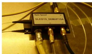
Fig. 5-5 Photograph of the SLED used for spectral slicing.
