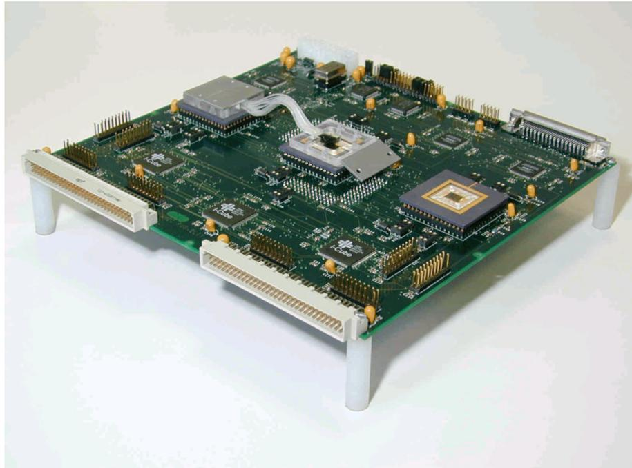
Figure 2.5: A guided-wave optical interconnect demonstrator: the OIIC system demonstrator.
