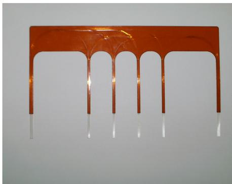
Figure 2.3: A flexible foil with optical fibres [29, 30]
