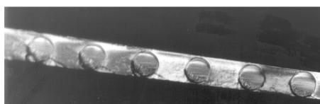
Figure 6.19: A cross section of a  $1 \times 8$  “embedded POF” array
