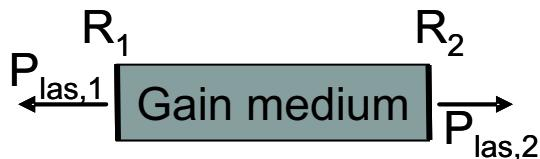
**Figure 3.1:** Schematic view of a semiconductor laser diode.
