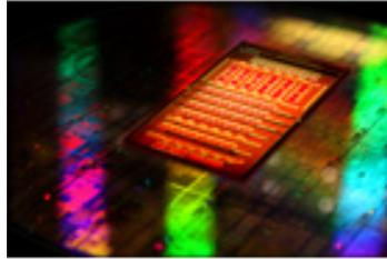
**Figure 1.3:** Prototype of a CMOS chip with an on-chip optical interconnect overlay (reproduced from [12]). Optical interconnects would allow to increase the information transfer rate and this transfer of large amounts of information would happen at higher speeds and using less power than using current electronic interconnects
