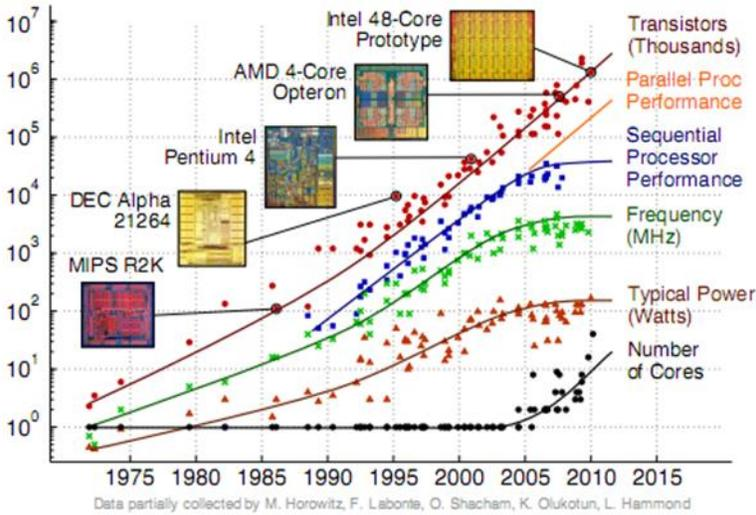
**Figure 1.1:** Illustration of increases in the numbers of transistors following Moore’s law, and corresponding evolutions of the clock-rate and performance. The figure is reproduced from the ref [3].
