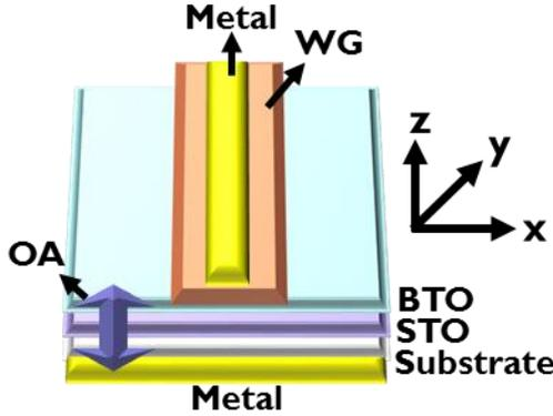
**Figure A.2:** The schematic of the Si-integrated waveguide using the c-oriented BTO and vertical electrode configuration.
