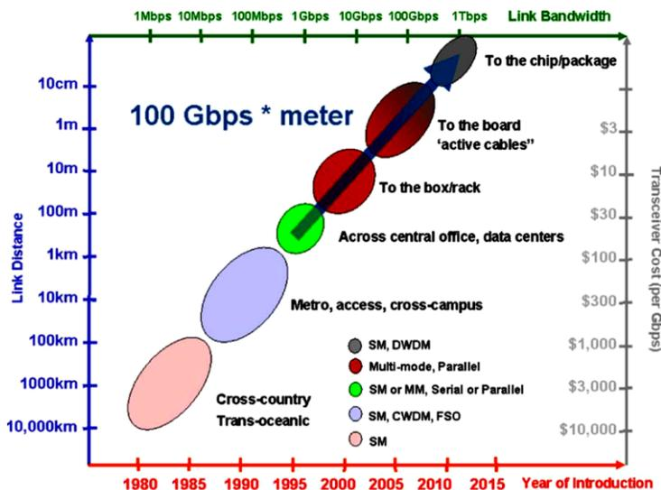
**Figure 1.4:** Chronological roadmap for the introduction of optical interconnects in digital systems, describing the link distance versus link bandwidth and cost. The figure is reproduced from the ref. [7].
