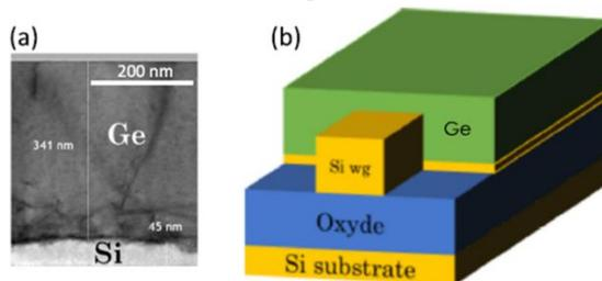
**Figure 1.10:** The cross-sectional TEM for Ge epitaxy on Si and the device schematic of the Ge photodetectors. The figure is reproduced from the ref. [25].
