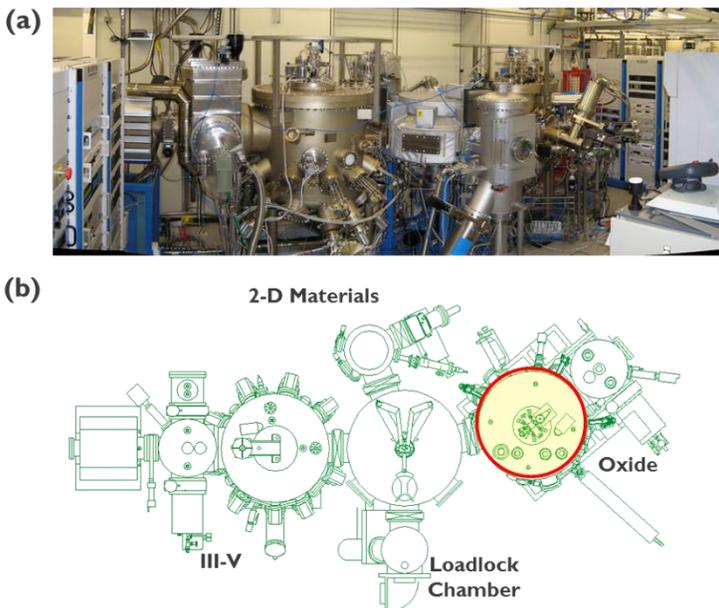
**Figure 2.5:** (a) Photograph and (b) schematic diagram of the Riber49 200mm MBE cluster system.
