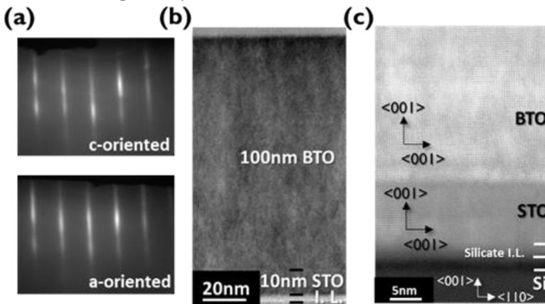
**Figure 5.8:** (a) The RHEED patterns for c- and a-oriented BTO layers on Si(001). TEM (b) and HAADF-STEM (c) images for 100-nm-thick layers of a-oriented BTO on a Si(001) substrate with a 10-nm-thick STO buffer layer.
