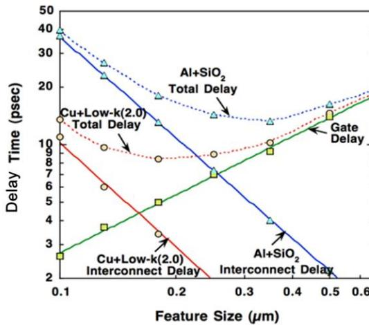
**Figure 1.2:** Delay time as a function of the feature size of the gate length in transistors using copper/low-k(2.0) and Al/SiO<sub>2</sub>. The figure is reproduced from the ref. [5].
