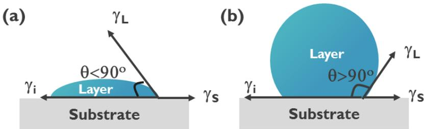
**Figure 2.4:** (a) Hydrophilic and (b) hydrophobic surfaces corresponding to layer-by-layer and island growth modes, respectively.
