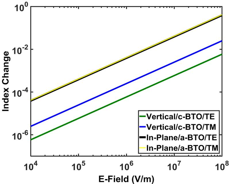
**Figure 5.2:** The index modulations in functions of the electric field for different device schemes described in Figure 5.1. For the a-oriented BTO, the angle between the domain and the electric field  $\phi=45^\circ$ .
