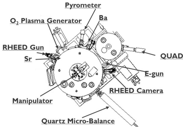
**Figure 2.6:** Components of the oxide chamber.
