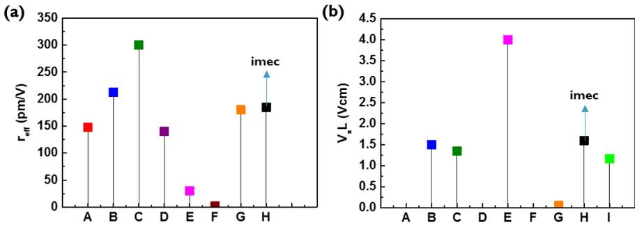
**Figure 6.25:** Benchmarks of the (a)  $r_{\text{eff}}$  and (b)  $V_{\pi}L$ , which are derived in different hybrid Si-based materials and their optical modulators. A: BTO/Si from [17]. B: BTO/Si [1]. C: BTO/Si [4]. D: BTO/Si [18]. E:  $\text{LiNbO}_3/\text{Si}$  [11]. F:  $\text{Si}_3\text{N}_4/\text{Si}$  [19]. G: Organic polymer/Si [20]. H: this work. I: PZT/Si [21]
