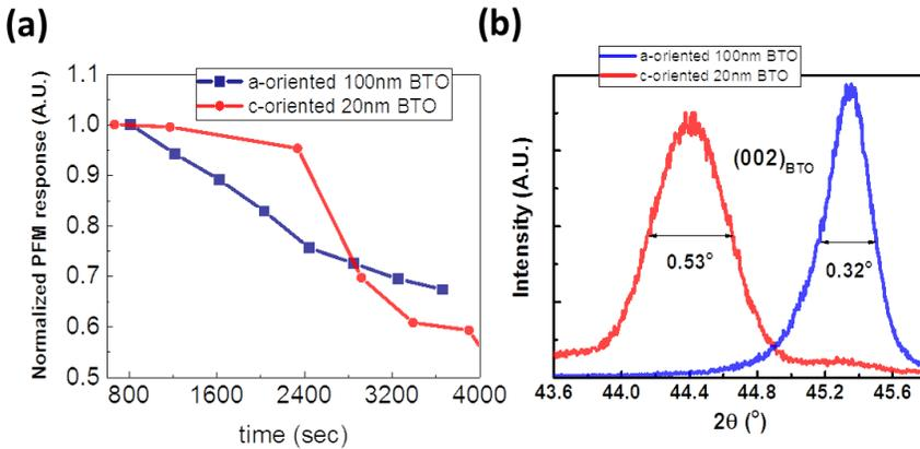
**Figure 6.21:** (a) The comparisons of the polarization stability between a-oriented 100 nm BTO and c-oriented 20 nm BTO. (b) The  $\omega$ - $2\theta$  scan for the a-oriented 100 nm BTO and c-oriented 20 nm BTO.
