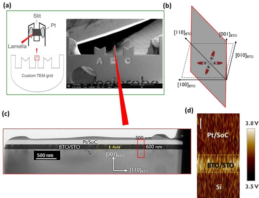
**Figure 6.19:** (a) The custom TEM grid to place the TEM lamella for the in-plane PFM. (b) The schematic illustrating that the TEM specimen is prepared along  $[001]_{\text{BTO}}$  and  $[110]_{\text{BTO}}$  by the FIB. The in-plane BTO domains show orientations along  $[100]_{\text{BTO}}$ ,  $[-100]_{\text{BTO}}$ ,  $[010]_{\text{BTO}}$  and  $[0-10]_{\text{BTO}}$ . (c) The TEM lamella for the in-plane PFM (d) The PFM amplitude after the 1-hour poling by -3 V.
