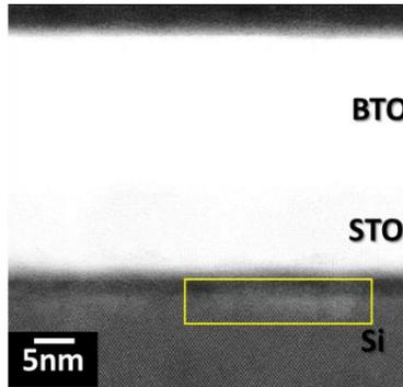
**Figure 4.8:** The HAADF-STEM for as-deposited 20 nm BTO on a Si(001) substrate using a 10 nm STO buffer. The image is presented with high brightness and contrast to indicate the Si region.
