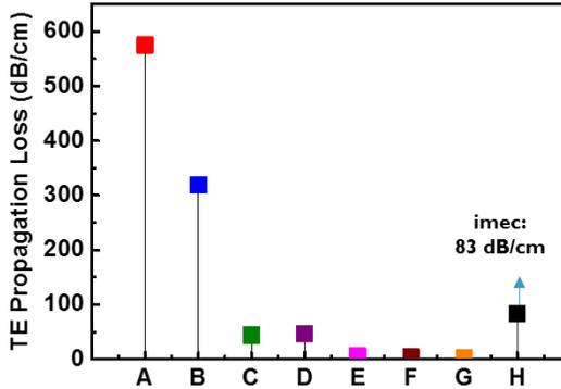
**Figure 6.24:** Benchmarks of the propagation loss for different BTO-based TE-mode waveguides. A: BTO/Si [14]. B: BTO/Si [14]. C: BTO/Si [1]. D: BTO/Si [4]. E: BTO/Si [2]. F: BTO/MgO [15]. G: Si [16]. H: this work.
