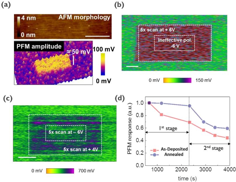
**Figure 4.12:** (a) The AFM morphology and PFM response mapping for as-deposited BTO. The square area in the PFM image is written by DC +6 V with 5 scans. The PFM response mapping of (b) as-deposited and (c) annealed BTO with different poling bias values. Scale bars represent 500 nm. (d) The time evolution of the PFM response for as-deposited and annealed BTO polarized by +6 V with 5 scans.
