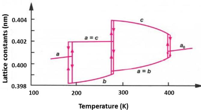
**Figure 1.21:** Lattice constants  $a$  and  $c$  as a function of temperature. The figure is reproduced from the ref. [63].
