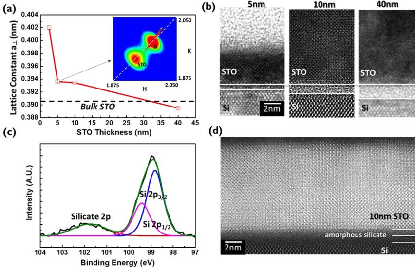
**Figure 5.3:** (a) The lattice constant  $a_{\perp}$  as a function of the STO layer thickness on a Si(001) substrate. The inset shows the RSM of  $(220)_{\text{Si}}$  for a 5-nm-thick STO layer. (b) HRTEM of 5-, 10-, and 40-nm-thick layers of STO on Si(001). (c) A Si 2p XPS scan of the 5-nm-thick STO layer on Si(001). (d) HAADF-STEM of a 10-nm-thick STO layer on Si(001)
