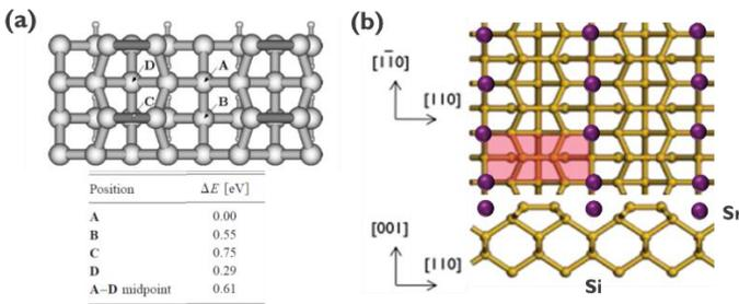
**Figure 4.2:** (a) Map of surface potential energy for a Sr atom on a Si(001) surface with 1x2 reconstruction. The figure is reproduced from the ref. [13]. (b) Schematic of Sr atoms on Si(001) surface to form 1x2 reconstruction.
