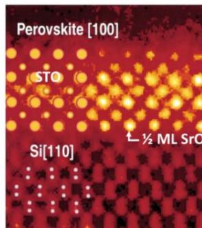
**Figure 1.24:** Z-contrast image of SrTiO<sub>3</sub> on (001) silicon. The figure is reproduced from the ref. [78].
