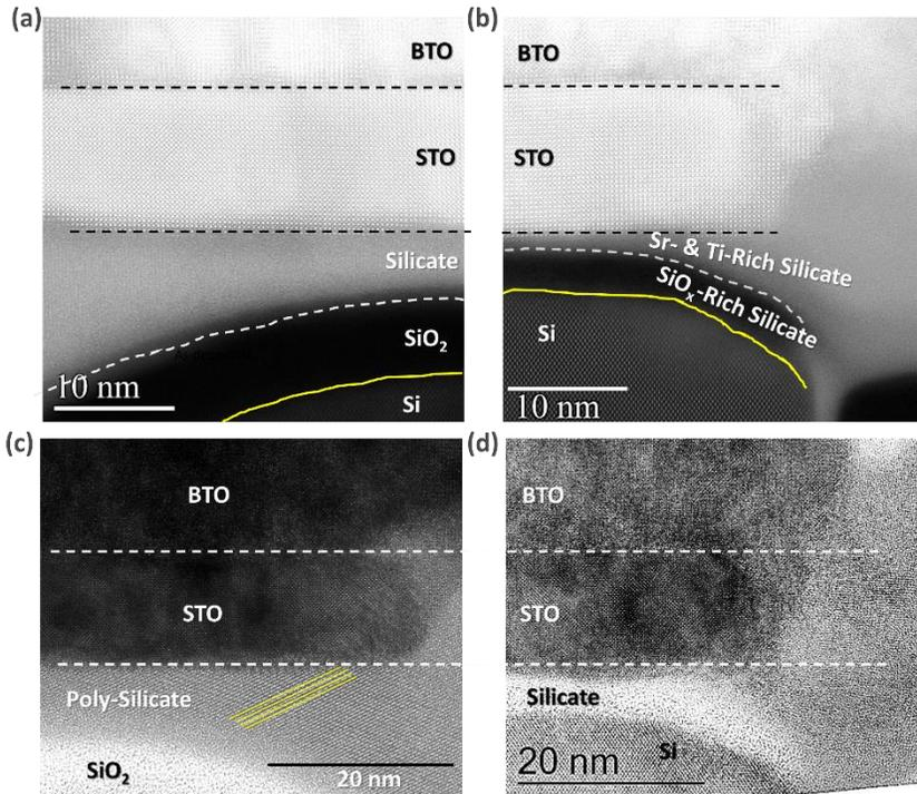
**Figure 6.8:** The HAADF-STEM images of (a) oxygen-annealed and (b) as-deposited samples. The HR-TEM images of (c) oxygen-annealed and (d) as-deposited samples.
