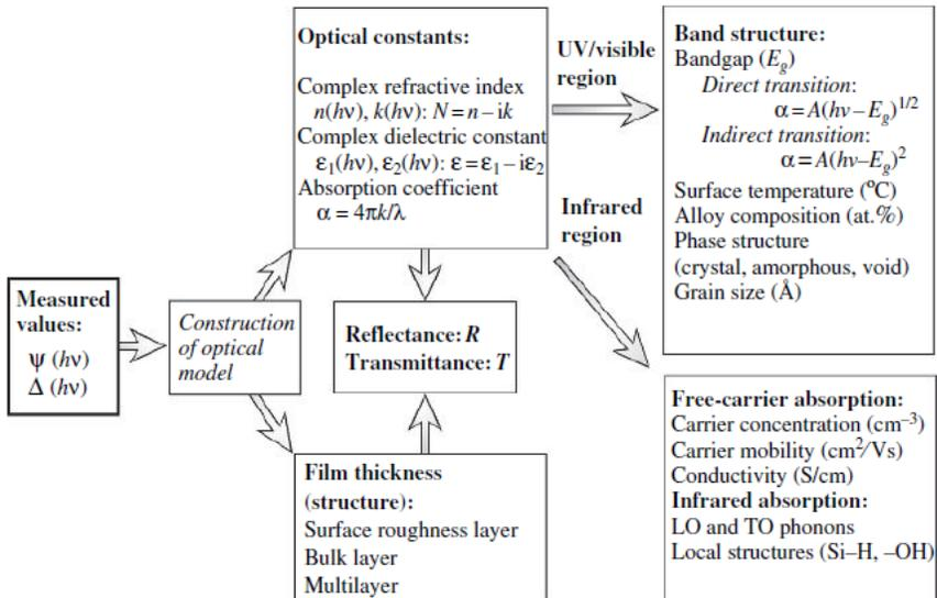
**Figure 2.14:** Flow chart describing characterization of physical properties by SE. This figure is reproduced from the ref. [13].
