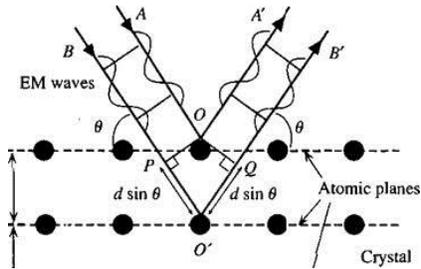
**Figure 2.10:** Schematic of Bragg's condition. The figure is reproduced from the ref. [11].
