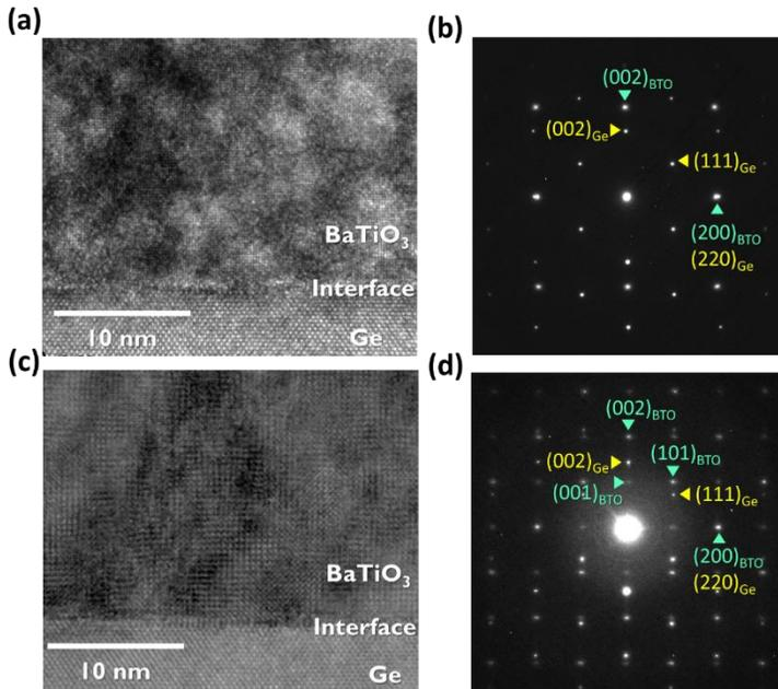
**Figure 3.8:** (a) and (b) are HR-TEM and SAED images of sample A with 90% [Ti] respectively; (c) and (d) are those images for sample B with 4% extra [Ti]. The miller planes in the SAED images are indexed based on the tetragonal lattice system and Ge(001) reference
