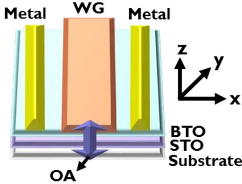
**Figure A.3:** The schematic of the Si-integrated waveguide using the c-oriented BTO and in-plane electrode configuration.
