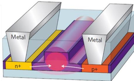
**Figure 1.12:** Cross-section of the device structure implementing the carrier injection mechanism. Highly doped p- and n-regions are separated by an ‘intrinsic region’ in which the waveguide is formed. Forward-biasing the device causes free electrons and holes to be injected into the ‘intrinsic’ waveguide region. The figure is reproduced from the ref. [33].
