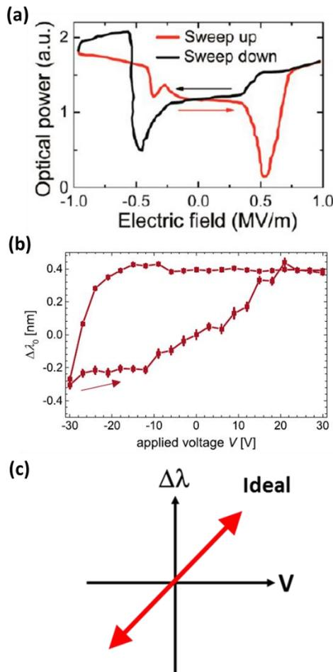
**Figure 6.11:** The (a) optical power and (b) spectral shift as a function of the applied electric field and voltage. These figures are reproduced
