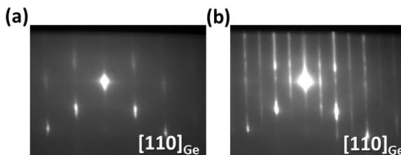
**Figure 3.1:** RHEED patterns along  $[110]_{\text{Ge}}$  for  $\text{Ge}(001)$  substrate (a) with and (b) without native oxide.
