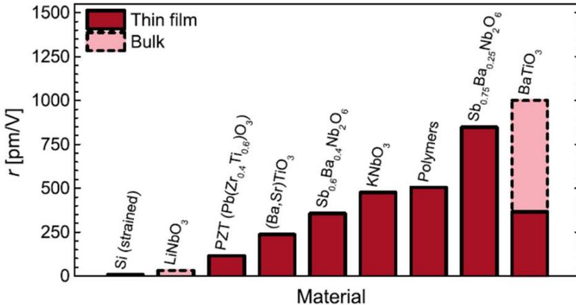
**Figure 1.17:** Comparison of the effective Pockels coefficients  $r$  of common bulk and thin-film nonlinear materials. The figure is reproduced from the ref. [52-55]: BTO exhibits one of the largest Pockels coefficients of all
