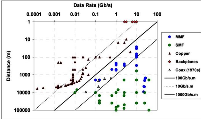
**Figure 1.5:** Data rate versus distance for commercial electrical versus optical links. The figure is reproduced from the ref. [7].
