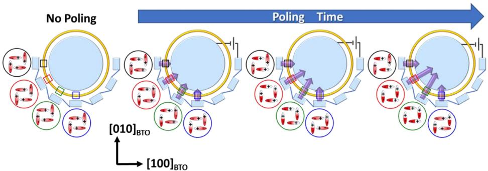
**Figure 6.16:** The time-evolved microscopic views of the BTO domains response with respect to the applied electric field at different regions of  $\phi=0^\circ$ ,  $30^\circ$ ,  $60^\circ$  and  $90^\circ$ . The purple arrow represents the domain polarization and the arrow length stands for the polarization strength in the macroscopic views. The gradient color for each dipole reveals the polarization strength in the microscopic views.
