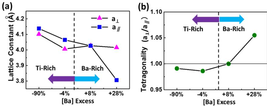
**Figure 3.7:** (a) The in-plane ( $a_{\parallel}$ ) and out-of-plane ( $a_{\perp}$ ) lattice constants, derived from  $\omega$ -2 $\theta$  scans shown in Figure 3.5. (b) The corresponding tetragonality ( $a_{\perp}/a_{\parallel}$ ) for all samples
