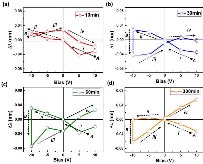
**Figure 6.14:** The bias-dependent spectral shift via the bias-sweeping mode 1 with the poling time  $T_1=T_2$  varying from (a) 10, (b) 30, (c) 60, and (d) 300 minutes.
