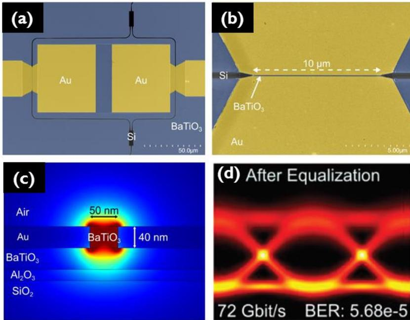
**Figure 1.19:** (a) and (b) Scanning electron microscopy (SEM) of the BTO/Si hybrid plasmonic modulator. (c) Simulated mode profile of the device. (d) Eye diagram of the data transmission. These figures are reproduced from the ref. [57].
