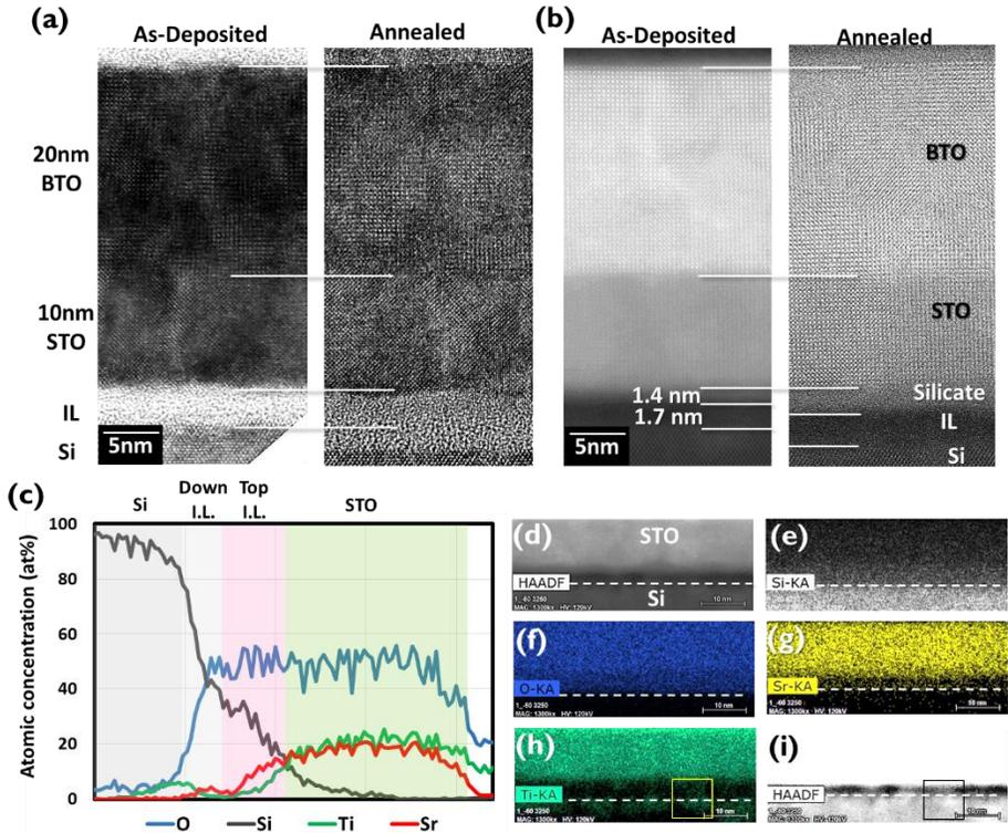
**Figure 4.6:** (a) HR-TEM and (b) HAADF-STEM images of as-deposited and annealed BTO samples. (c) Spatial atomic concentration for the annealed BTO (d) HAADF-STEM image with EDS analysis. EDS detection results for (e) Si (f) O (g) Sr and (h) Ti. (i) The HAADF-STEM image with different brightness and contrast from (d).
