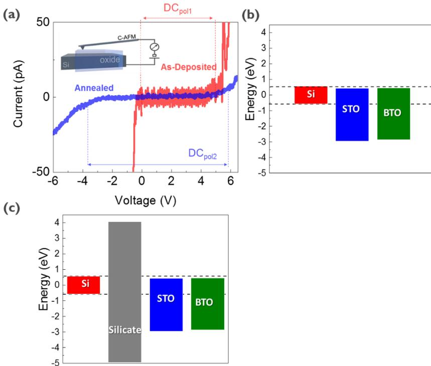
**Figure 4.11:** (a) The I-V measured by CAFM for as-deposited and annealed samples. The band diagram of (b) BTO/STO/Si and (c) BTO/STO/Silicate/Si heterostructure.
