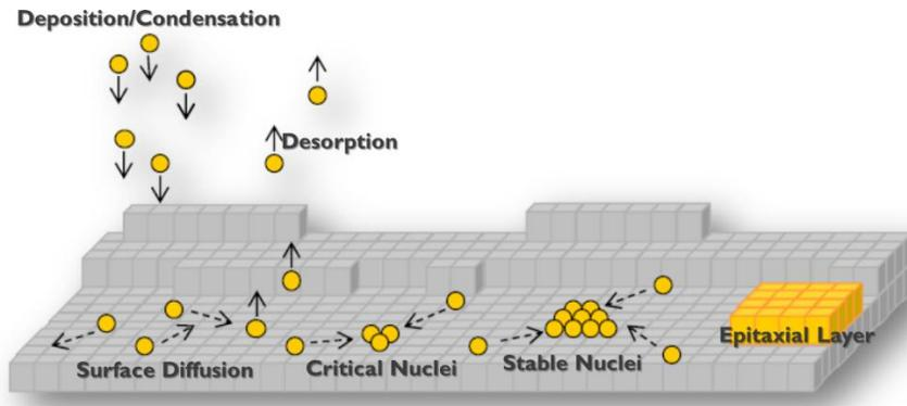
**Figure 2.2:** Atomic process of nucleation and epitaxy. The figure is reproduced from the ref. [2]
