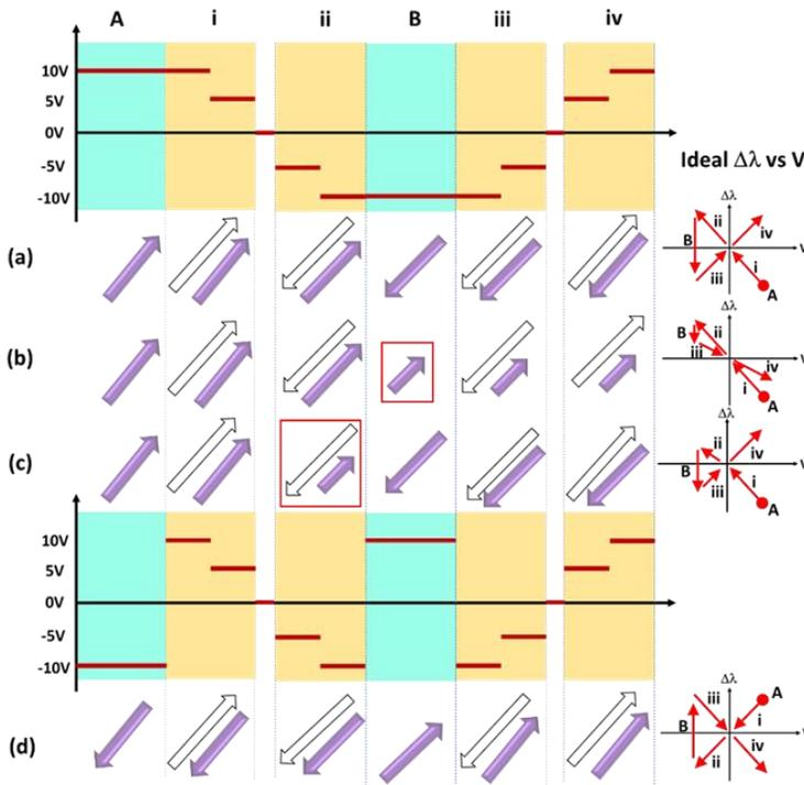
**Figure 6.17:** The macroscopic EO response to the interaction between the applied electric field and BTO domain polarization at different measurement steps. (a) The ideal situation for the bias-sweeping
