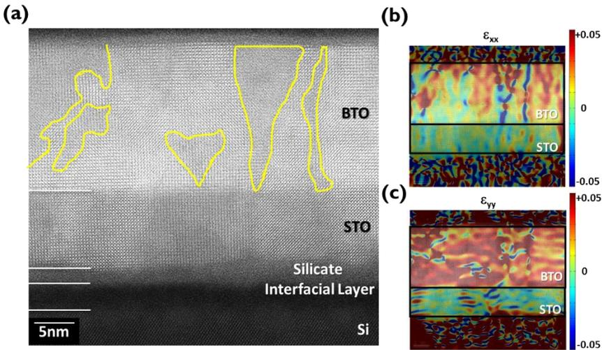
**Figure 4.10:** (a) HAADF-STEM of the annealed sample highlighted with detectable domain boundaries. The mappings of (b) in-plane ( $\epsilon_{xx}$ ) and (c) out-of-plane ( $\epsilon_{yy}$ ) strains obtained from GPA analysis.
