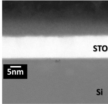
**Figure 4.7:** The HAADF-STEM for 10 nm STO on a Si(001) substrate with high brightness and contrast to indicate the Si region.
