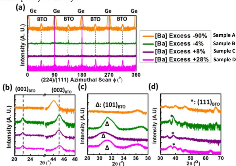
**Figure 3.5:** (a) The azimuthal  $\phi$  scan of  $(\pm 1\pm 1)_{\text{BTO/Ge}}$  for the samples B to D, and that of  $(\pm 2\pm 2)_{\text{BTO/Ge}}$  for the sample A. The  $\omega$ - $2\theta$  scan along (b)  $[001]_{\text{BTO}}$ , (c)  $[101]_{\text{BTO}}$  and (d)  $[111]_{\text{BTO}}$  for all the samples.
