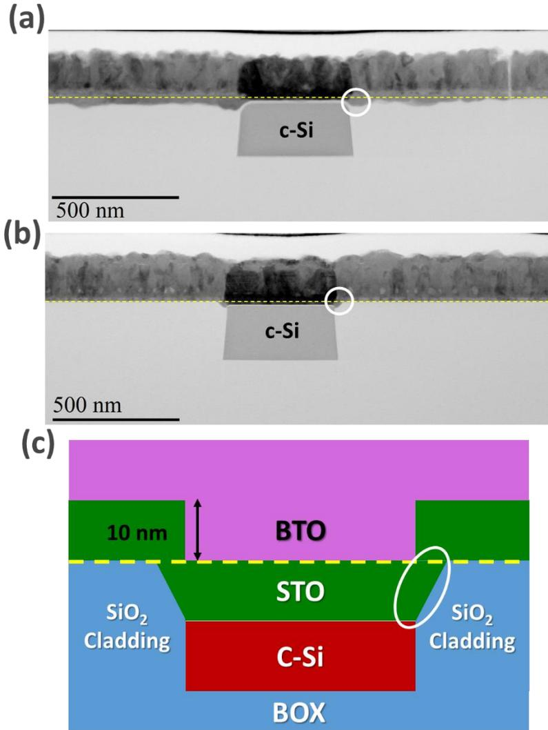
**Figure 6.7:** The ABF-STEM images of (a) oxygen-annealed and (b) as-deposited samples. (c) The structure schematic.
