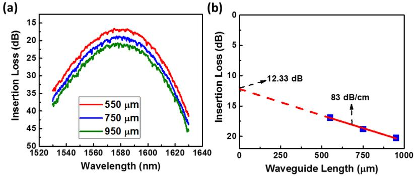
**Figure 6.5:** (a) The measured transmission spectra for the 550  $\mu\text{m}$ , 750  $\mu\text{m}$  and 950  $\mu\text{m}$  waveguides which are annealed with oxygen at 800  $^{\circ}\text{C}$  for 4 hours. (b) The linear regression of the insertion loss with waveguide length. The vertical intercept is -12.33 dB, which reveals the insertion loss of the grating coupler is 6.2 dB. The slope shows the waveguide propagation loss of 83 dB/cm.
