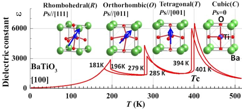
**Figure 1.22:** Dielectric constant, crystal structure, and spontaneous polarization as functions of temperature. The figure is reproduced from the ref. [64].
