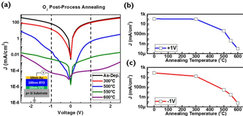
**Figure 5.9:** (a) The  $J$ - $V$  curves in terms of various post-process annealing temperatures under 30 min oxygen ambient for 100-nm-thick layers of a-oriented BTO on highly p-doped Si substrates with a 10 nm STO buffer layer. The top electrode is gold (10 nm). (b) and (c) are the current density at +1 V and -1 V, respectively, for different annealing temperatures.
