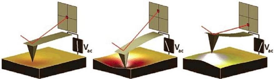
**Figure 2.16:** Illustration of PFM operation. The sample deforms in response to the applied voltage. This, in turn, causes the cantilever to deflect, which can then be measured and interpreted in terms of the piezoelectric properties of the sample. These figures are reproduced from the ref. [15].
