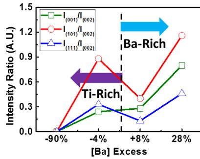
**Figure 3.6:** The XRD intensity ratio of  $(001)_{\text{BTO}}$ ,  $(101)_{\text{BTO}}$  and  $(111)_{\text{BTO}}$  to  $(002)_{\text{BTO}}$  for all samples, evaluated from the  $\omega$ -2 $\theta$  scans shown in Figure 3.5.
