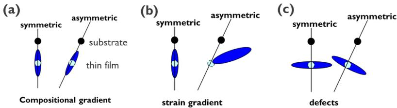
**Figure 2.12:** Relationships between layer and substrate in RSM illustrating the effect of (a) a compositional gradient, (b) a strain gradient, and (c) defects. The green dot-like signals indicate the ideal crystallinity in the thin film. However, different imperfect properties makes the signal become an ellipse and show different tilt angles as well as positions. These figures are reproduced from the ref. [12].
