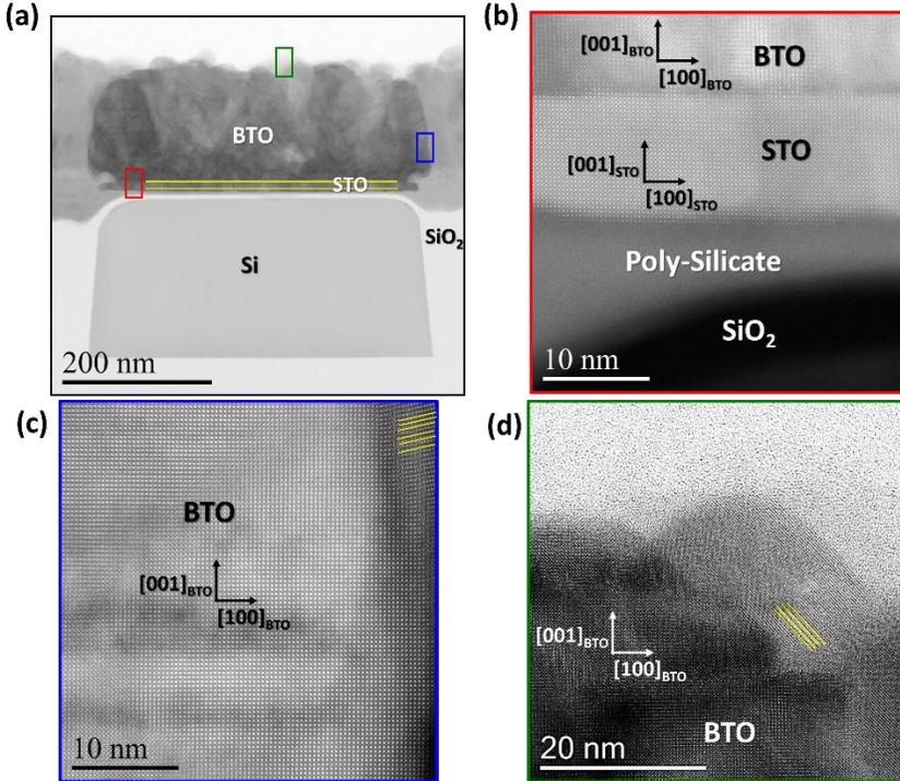
**Figure 6.10:** (a) The ABF-STEM of the oxygen-annealed sample. The different locations for zoom-in analysis are labelled on the BTO/STO on the crystalline Si waveguide region. (b) The HAADF-STEM image at the bottom-right BTO. (c) The HAADF-STEM image at the right edge of the BTO and (d) The HR-TEM at the top of the BTO.
