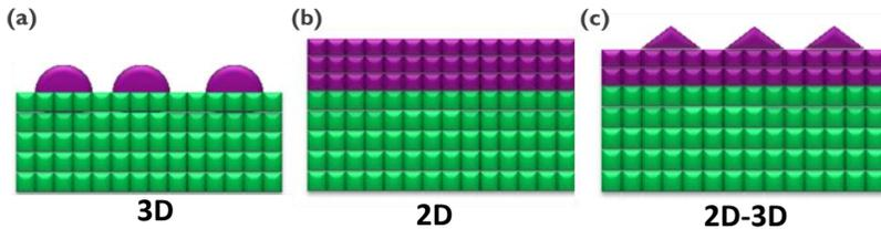
**Figure 2.3:** Three modes of thin-film growth: (a) Volmer-Weber (island growth), (b) Frank-van der Merwe (layer-by-layer growth), and (c) Stranski-Krastanov. These figures are reproduced from the ref. [3].
