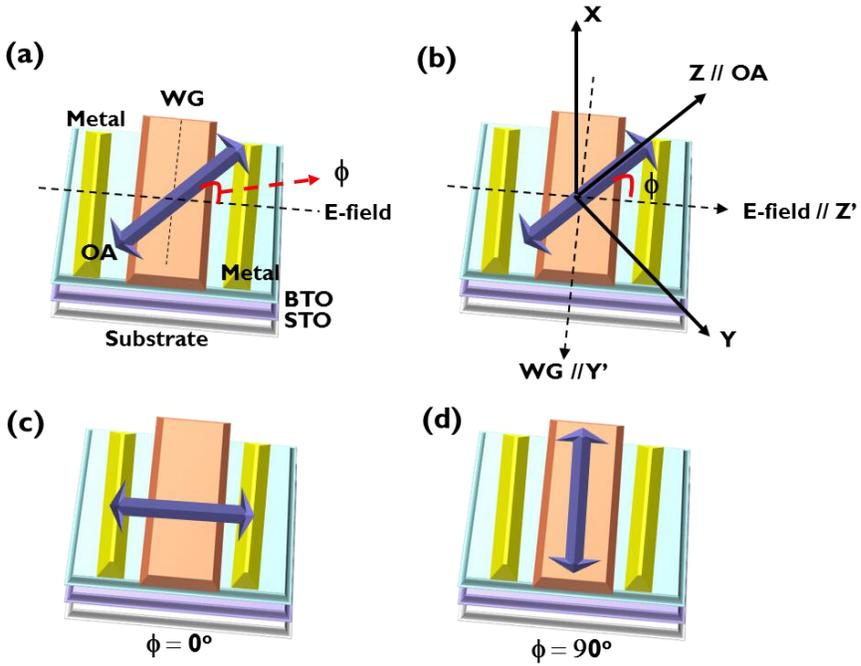
**Figure A.5:** (a) The schematic of the Si-integrated waveguide using the a-oriented BTO and in-plane electrode configuration. (b) The definitions for the x-y-z- and x-y'-z' coordinates. The device when (c)  $\phi=0^\circ$  and (d)  $\phi=90^\circ$
