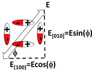
**Figure 6.22:** Relationship between the applied electric field and domains.
