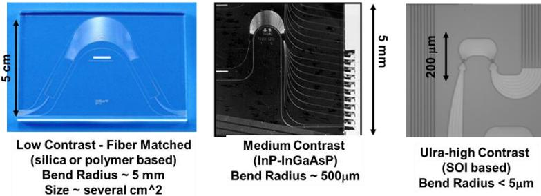
**Figure 1.9:** The effect of the index contrast between the core and cladding on the bending radius. The figure is reproduced from the ref. [18].
