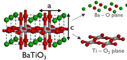
**Figure 1.20:** BTO perovskite crystal structure, with lattice constants  $a$  and  $c$ .
