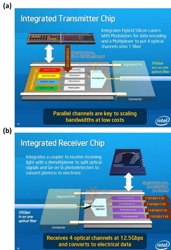
**Figure 1.8:** Schematic for 50 Gb/s transmitter and receiver chips from Intel. The figure is reproduced from the ref. [17].
