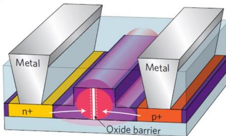
**Figure 1.13:** Cross-section of the device structure implementing the carrier accumulation mechanism. A thin insulating layer of  $\text{SiO}_2$  is used to isolate two halves of the waveguide to form a capacitor structure. The figure is reproduced from the ref. [33].
