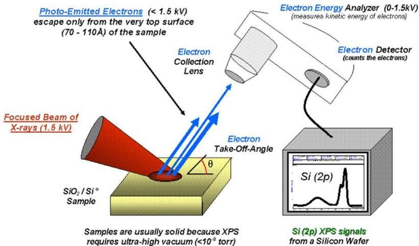
**Figure 2.18:** Basic components of the monochromatic XPS system. These figures are reproduced from the ref. [16].
