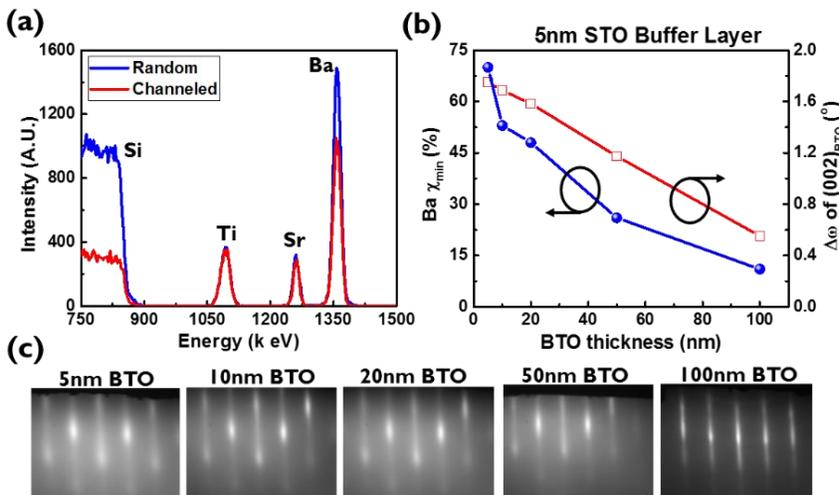
**Figure 5.5:** (a) The RBS spectra for a 5-nm-thick BTO layer with a random or channeled configuration on a 5-nm-thick STO layer on a Si substrate. (b) Ba  $\chi_{\min}$  for RBS channeling and FWHM of the (002)<sub>BTO</sub> rocking
