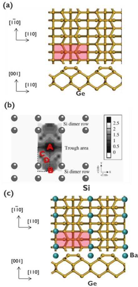
**Figure 3.2:** (a) Schematic of 1x2 reconstructed Ge surface with dimers (b) Map of surface potential energy for a Ba atom on a Si(001) surface. The figure is reproduced from the ref. [30]. (c) Schematic of Ba atoms on Ge(001) surface to form 1x2 reconstruction.
