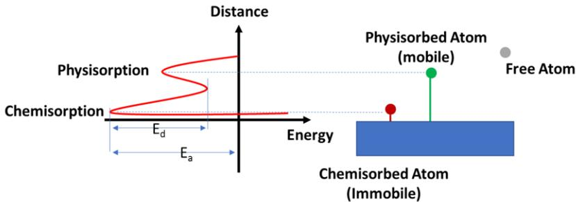
**Figure 2.1:** Physicochemical interactions between adatoms from vapor and substrate surface. The figures are reproduced from the ref. [2].
