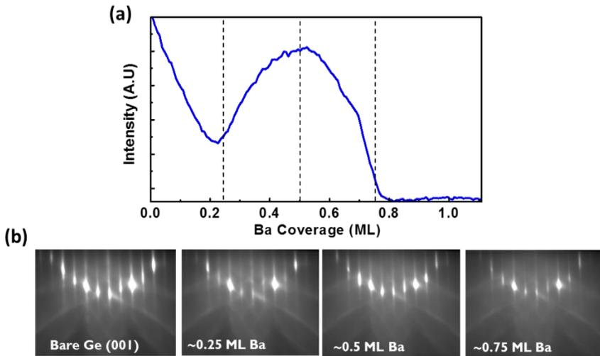
**Figure 3.3:** (a) The RHEED intensity for 1/2-order streak line as function of Ba coverage (b) corresponding RHEED patterns.
