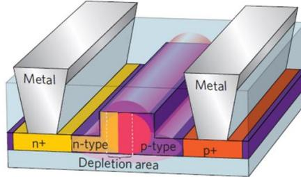
**Figure 1.14:** Cross-section of the device structure implementing the carrier depletion mechanism. Lightly doped p- and n-type regions abut in the waveguide to form a p-n diode. The depletion area of the diode becomes larger with increasing reverse bias voltage. The figure is reproduced from the ref. [33].
