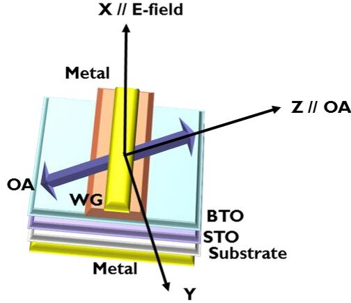
**Figure A.4:** The schematic of the Si-integrated waveguide using the a-oriented BTO and vertical electrode configuration.
