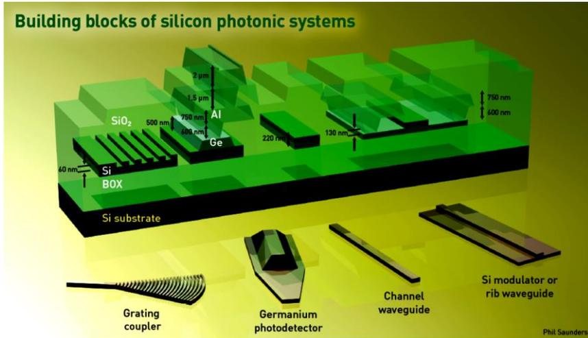
**Figure 1.7:** Schematic for building blocks of silicon photonic systems. The figure is reproduced from the ref. [16].
