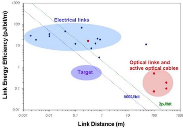
**Figure 1.3:** Energy per bit per meter versus the maximum reach of the link. The figure is reproduced from the ref [7].
