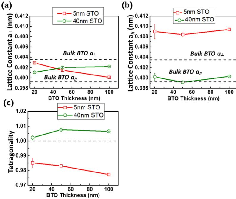
**Figure 5.6:** (a) The  $a_{\perp}$ , (b)  $a_{\parallel}$ , and (c) tetragonality of BTO films with different thicknesses on 5- and 40-nm-thick STO buffer layers.
