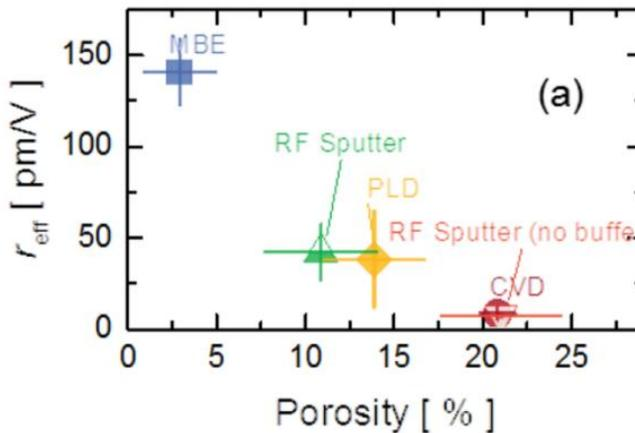
**Figure 1.26:** Effective Pockels coefficient  $r_{\text{eff}}$  for BTO vs porosity using different deposition techniques. The figure is reproduced from the ref. [84].
