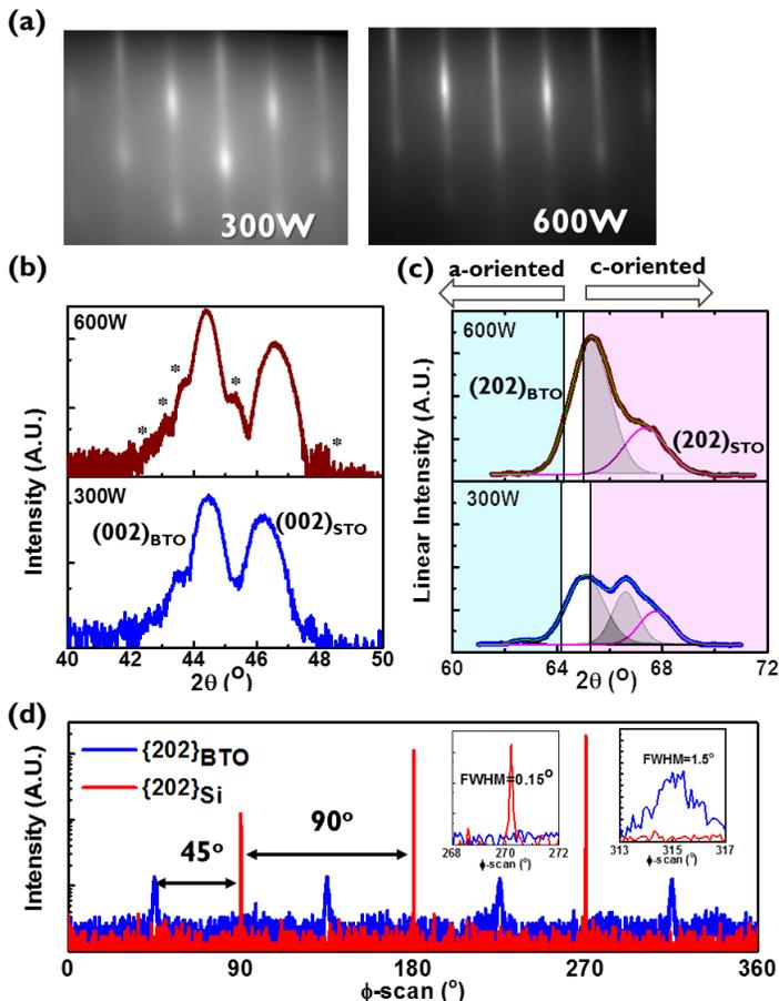
**Figure 4.5:** (a) RHEED patterns for BTO prepared at 630 °C with 300 W and 600 W. (b) The  $\omega$ -2 $\theta$  scans of (002)<sub>BTO/STO</sub> for samples prepared at 300 W and 600 W. (c) The  $\omega$ -2 $\theta$  scans of (202)<sub>BTO/STO</sub> for samples prepared at 300 W and 600 W. (d) The  $\phi$ -scan of {202}<sub>BTO/Si</sub> for the sample prepared at 600 W. Insets show magnifications of the BTO and Si peaks and their corresponding FWHM.
