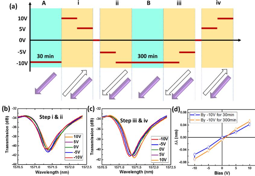
**Figure 6.18:** (a) The bias-sweeping plan with -10 V for 30 and 300 minutes at Step A and Step B respectively to obtain the linear EO condition. The transmission spectra collected in (b) Step i and Step ii and (c) Step iii and Step iv. (d) The measured spectral shift in function of bias showing the linear EO behavior.
