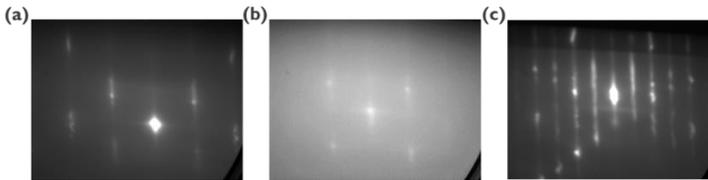
**Figure 4.1:** RHEED patterns along  $[110]_{Si}$  for Si(001) surface, which is covered with (a) native  $SiO_2$  (b) 2 monolayer Sr on the native oxide (c)  $\frac{1}{2}$  ML Sr.
