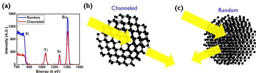
**Figure 2.19:** (a) The typical random and channeled RBS spectra for BTO on STO-buffered Si(001) substrate. The schematic of the (b) channeled and (c) random cases.
