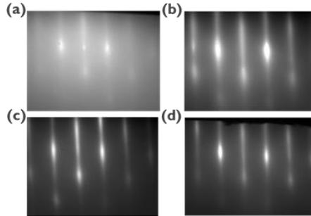
**Figure 4.3:** RHEED patterns along  $[100]_{\text{STO}}$  for (a) 6 ML (2.4 nm) STO which was deposited at 150 °C (b) 6 ML (2.4 nm) STO which was recrystallized at 550 °C (c) 12 ML (4.8 nm) STO after 2 times of deposition and recrystallization process. (d) 10 nm STO.
