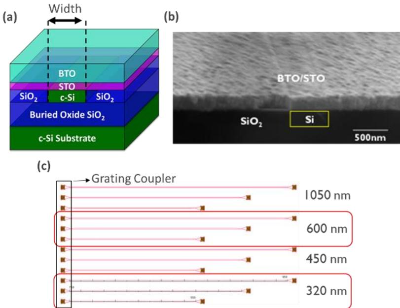
**Figure 6.3:** (a) The structure schematic of the hybrid BTO/Si waveguides. (b) The cross-sectional SEM image of the hybrid BTO/Si waveguides. (c) The waveguide arrays with the width of 320 nm,
