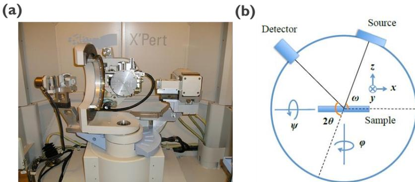
**Figure 2.11:** (a) A photograph of the equipment and (b) diagram describing all the angle definitions.
