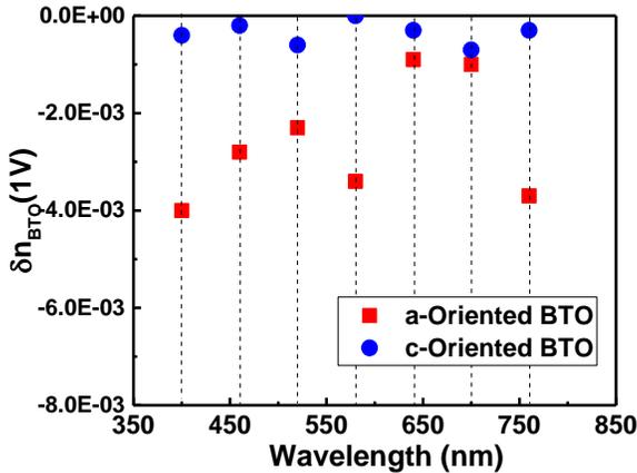
Figure 5.11:  $\delta n_{\text{BTO}}$  at 1 V for a- and c-oriented BTO.
