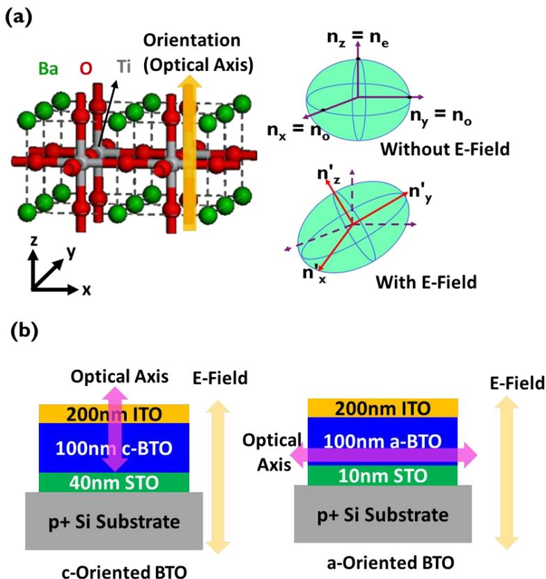
**Figure 5.12:** (a) Lattice structure for c-oriented BTO and its index ellipsoid without and with an applied electric field. (b) Relationship between the electric field and the optical axis in c- and a-oriented BTO.
