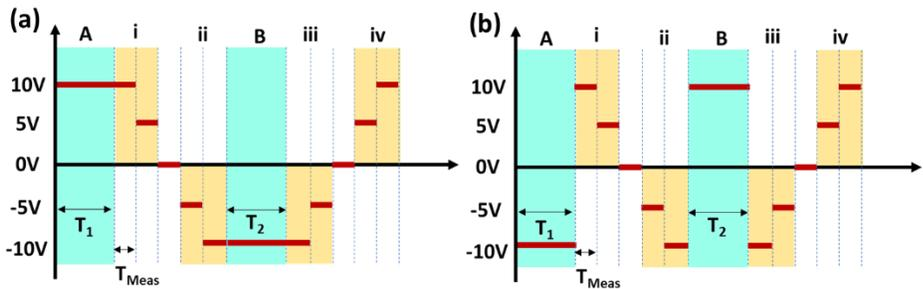
**Figure 6.13:** The bias steps for the (a) sweep mode 1 and (b) sweep mode 2.
