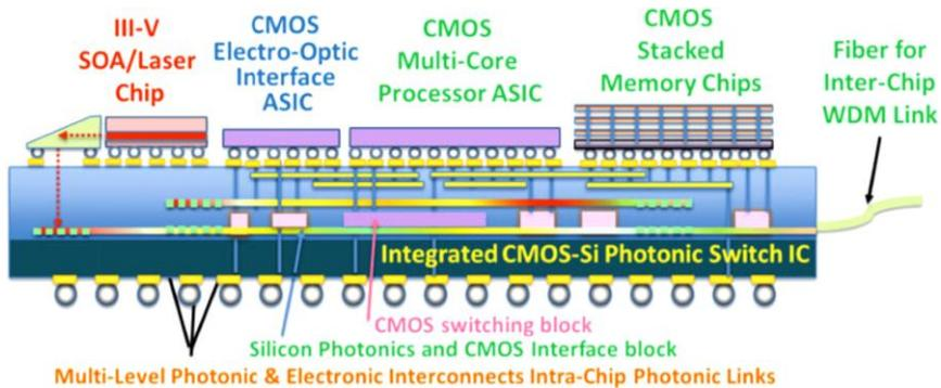
**Figure 1.6:** Schematic diagram of a possible compact terabit silicon photonics integrated circuit assembled with CMOS interface ICs, processor, stacked memory chips and III-V laser by heterogeneous integration technology. The figure is reproduced from the ref. [15].
