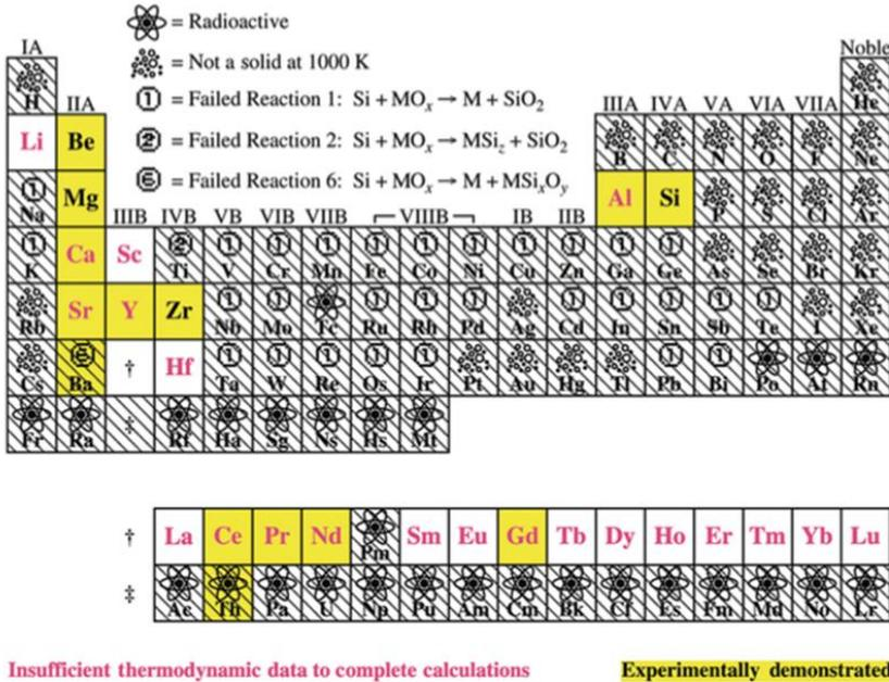
**Figure 1.25:** Thermo-dynamical stability of the oxides of elements in contact with Si at 1000K. The figure is reproduced from the ref. [79].
