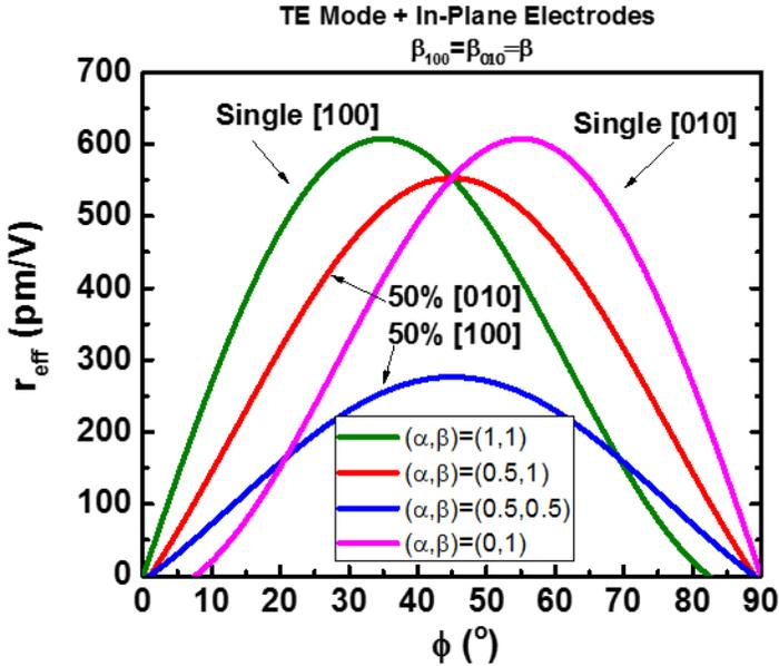
**Figure 6.1:** Calculated  $r_{\text{eff}}$  under different circumstances of domain randomness and domain orientations in the device for TE modulation.
