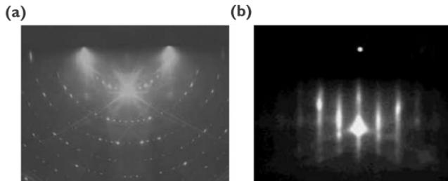
**Figure 2.8:** (a) Ideal and (b) typical RHEED patterns for 2-dimensional layers. [9]
