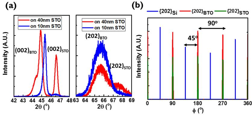
**Figure 5.7:** (a) The  $\omega$ - $2\theta$  XRD scans along  $[001]_{\text{BTO/STO}}$  and  $[101]_{\text{BTO/STO}}$  for a 100-nm-thick BTO layer on 10- and 40-nm-thick STO layer. (b) A  $\phi$ -scan of  $\{202\}_{\text{Si}}$ ,  $\{202\}_{\text{BTO}}$ , and  $\{202\}_{\text{STO}}$  for 100-nm-thick BTO on a 40 nm STO layer.
