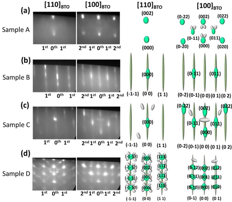
**Figure 3.4:** The RHEED diffraction patterns and corresponding schematics along  $[100]_{\text{BTO}}$  and  $[110]_{\text{BTO}}$  of (a) sample A with 90% extra [Ti], (b) sample B with 4% extra [Ti], (c) sample C with 8% additional [Ba] and (d) sample D with 28% additional [Ba], respectively.
