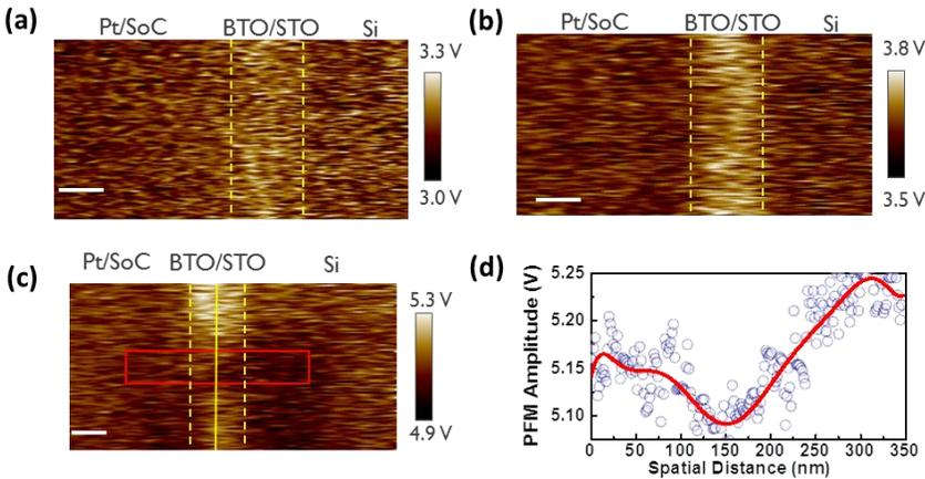
**Figure 6.20:** (a) The PFM amplitude for the un-poled sample. (b) The PFM amplitude for the sample poled by -3V for 1 hour. (c) The PFM amplitude for the sample being reversely poled by +4.5 V in the red rectangular area. (d) The sectional PFM amplitude along the yellow solid line in (c).
