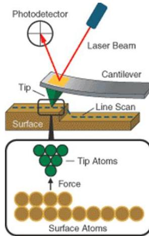
**Figure 2.15:** Schematic illustration of AFM. The figure is reproduced from the ref. [14].
