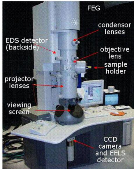
Figure 2.17: Major components of the TEM instrument.
