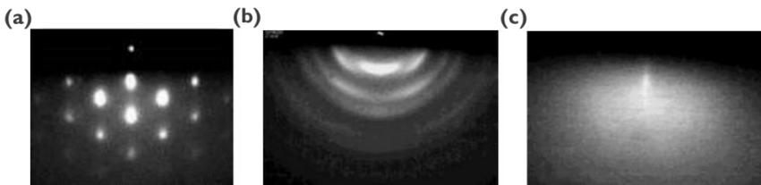
**Figure 2.9:** RHEED patterns for a (a) rough surface, (b) polycrystalline surface, and (c) amorphous surface. These figures are reproduced from the ref. [9].
