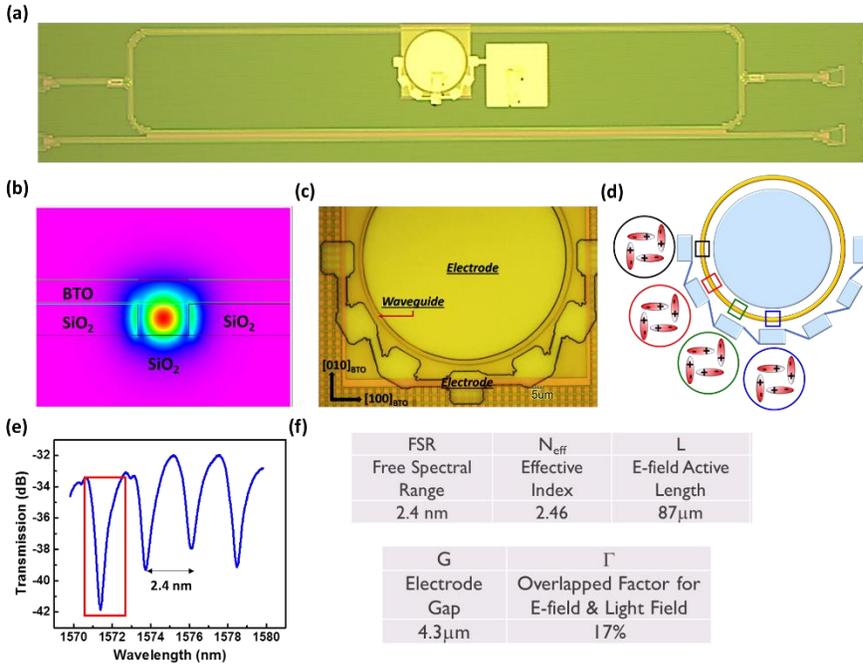
**Figure 6.12:** (a) The optical microscope image of the hybrid BTO/Si MZR modulator. (b) The mode distribution within the waveguide according to the finite element calculation. (c) The zoom-in image of the ring part. (d) The schematic of the a-oriented domains within the area between the central electrode pad and surrounding electrodes. (e) The transmission spectrum of the MZR modulator without bias. (f) Summary of the main design parameters for the hybrid BTO/Si MZR modulator.
