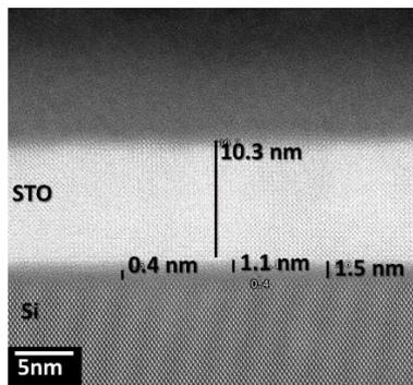
**Figure 4.9:** The HAADF-STEM for 10 nm STO on the Si(001) substrate.
