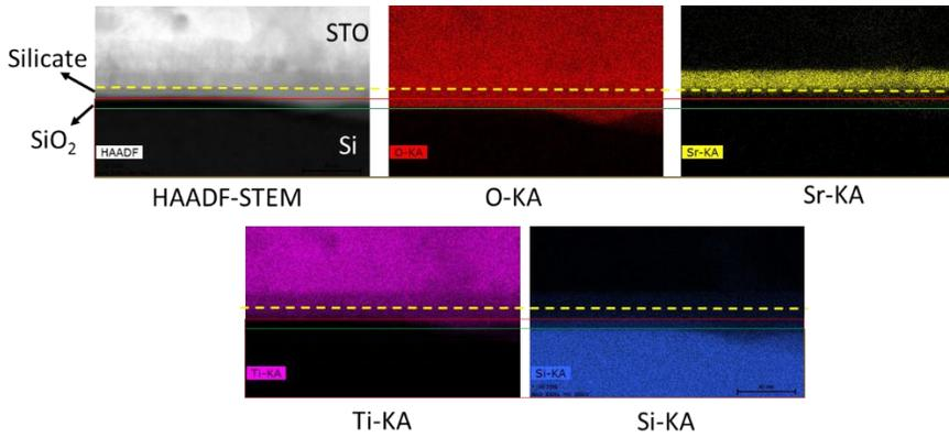
**Figure 6.9:** The EDS analysis at the STO/Si interface for the oxygen-annealed sample.
