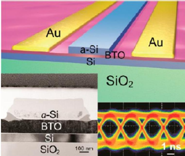
**Figure 1.18:** Schematic, transmission electron microscopy (TEM), and eye diagram of a BTO/Si hybrid optical modulator. These figures are reproduced from the ref. [56].
