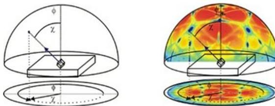
**Figure 2.13:** Schematic illustrating the construction of a pole figure by scanning  $\phi$  and  $\Psi$  in XRD. These figures are reproduced from the ref. [11].
