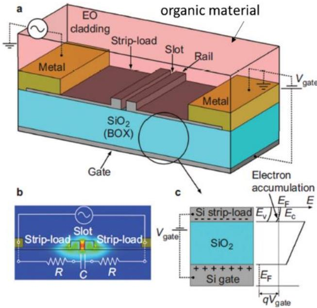
**Figure 1.16:** Schematic of the silicon-organic hybrid optical modulator. These figures are reproduced from the ref. [50, 51].
