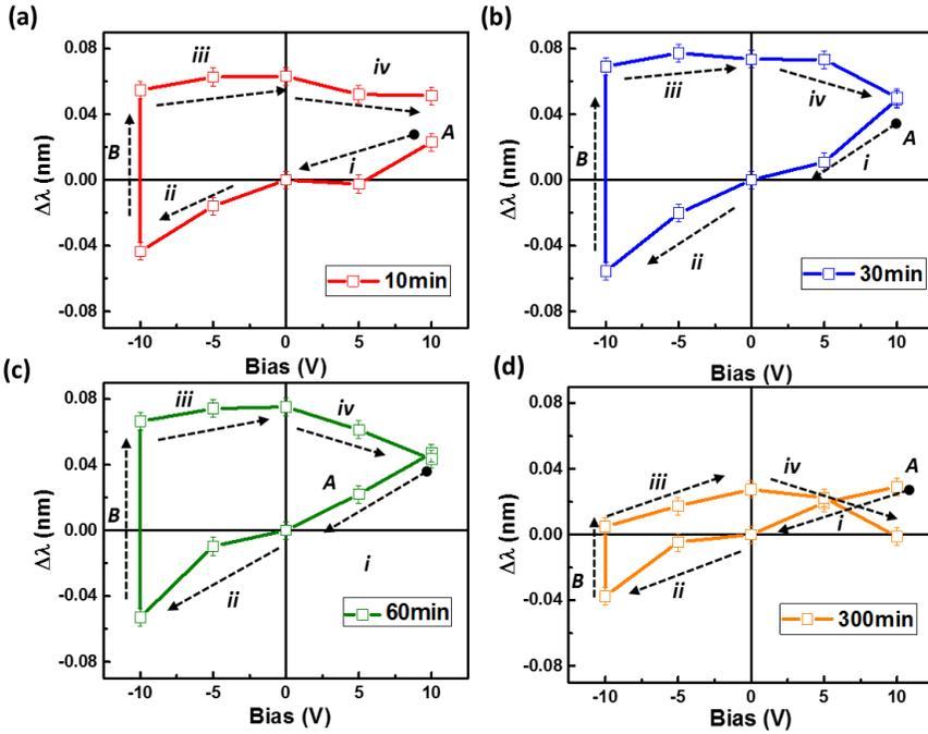
**Figure 6.15:** The bias-dependent spectral shift via the bias-sweeping mode 2 with the poling time  $T_1=T_2$  varying from (a) 10, (b) 30, (c) 60, and (d) 300 minutes.
