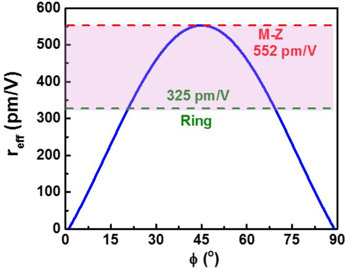
Figure 6.23: Evaluated ideal  $r_{\text{eff}}$  for the ring and mach-zehnder modulators.
