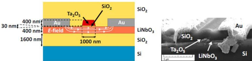
**Figure 1.15:** Schematic of the cross-section of the device structure and a scanning electron microscopy (SEM) image. These figures are reproduced from the ref. [49].
