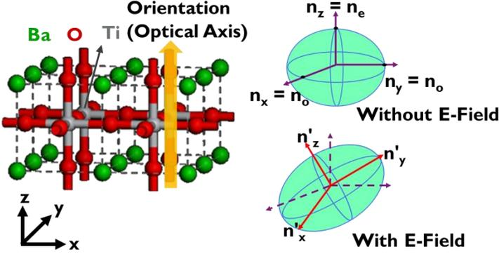
**Figure A.1:** Lattice structure for c-oriented BTO and its index ellipsoid without and with applied electric field.
