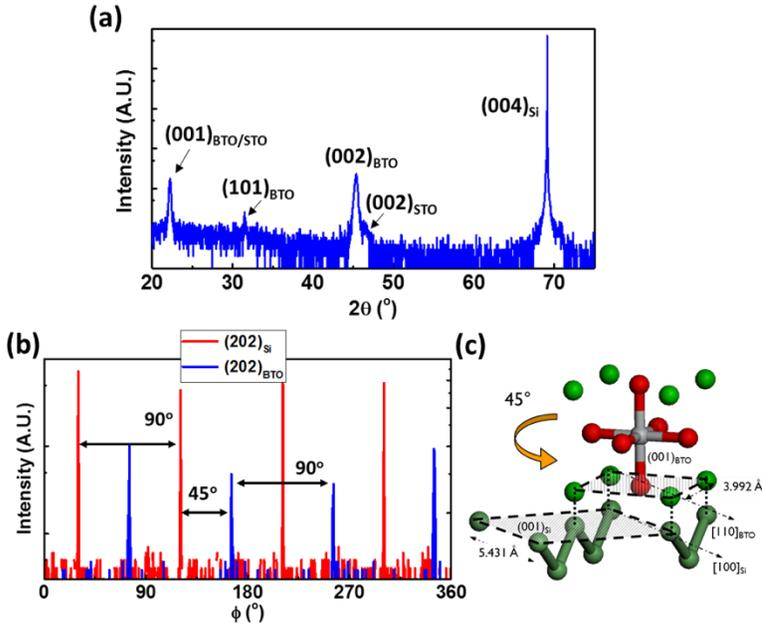
**Figure 6.6:** The (a)  $\omega$ - $2\theta$  and (b)  $\phi$ - scans of the sample annealed with oxygen at  $800^\circ\text{C}$  for 4 hours. (c) The schematic of the epitaxial relationship between BTO and Si(001).
