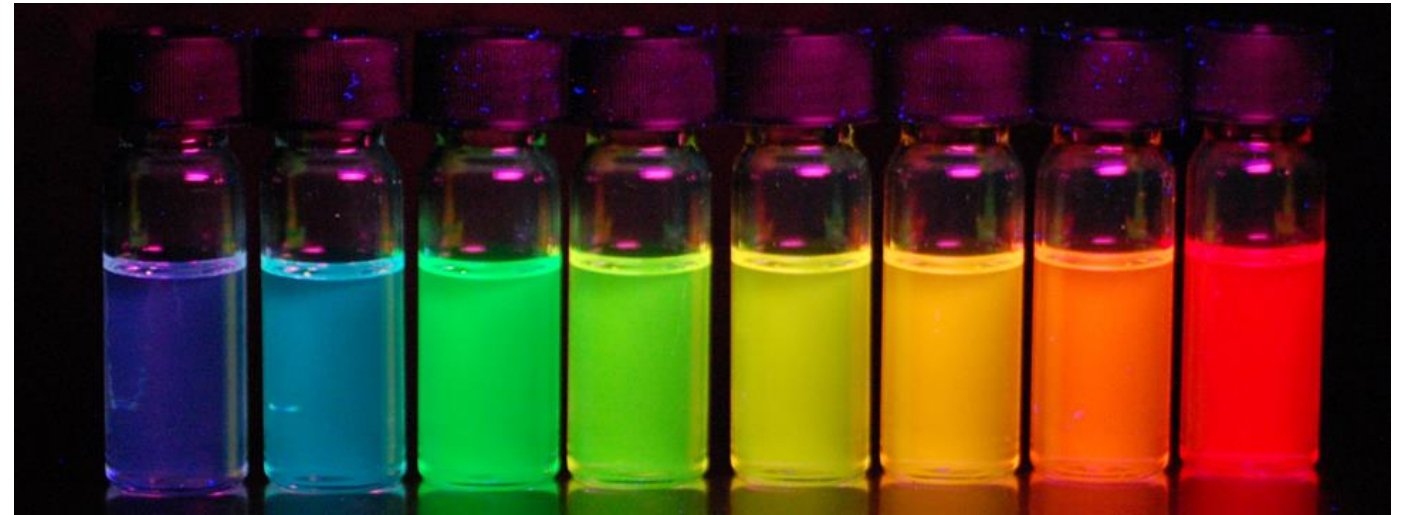
Spectral tunability through quantum confinement effect
