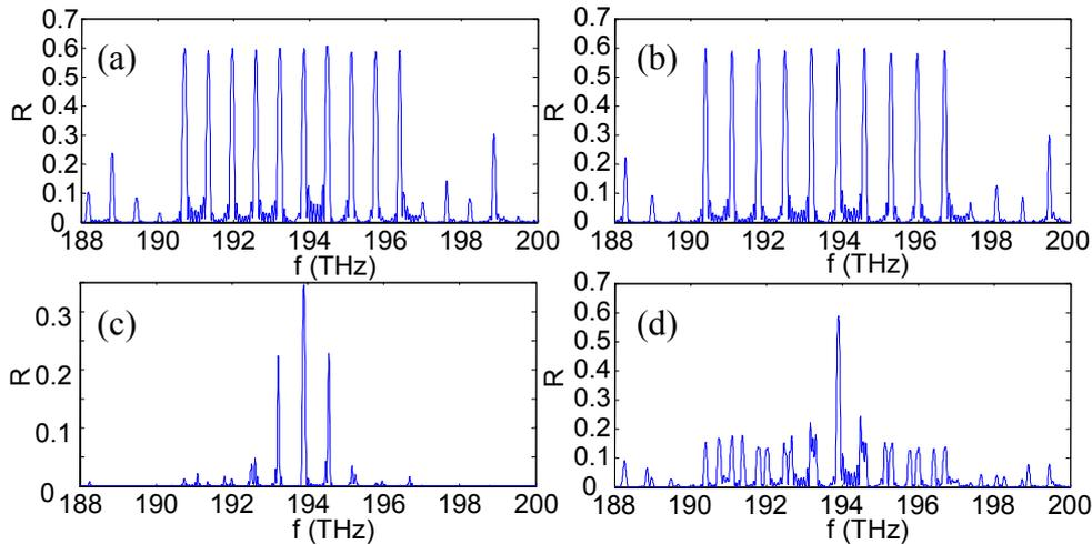
Figure 2. Power reflection spectra of (a) reflector 1 and (b) reflector 2, with 630 and 700GHz peak spacing respectively. (c) The product of the spectra,  $|r_1 r_2|^2$ , after a slight tuning of reflector 1 so that peaks 6 are aligned (SSG-DBR case). (d) Sum of the reflections,  $|r_1 + r_2|^2 / 4$ , (MGY case).
