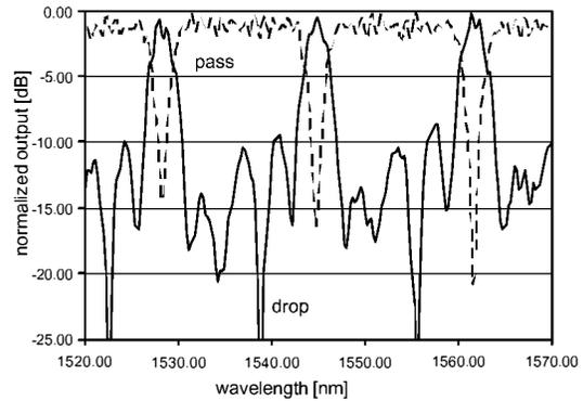
Fig. 4 Transmission characteristic of the five-stage CMZ from figure 3.
