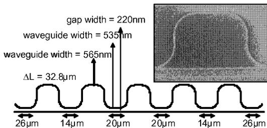
Fig. 3 Design of a 5-stage CMZ
