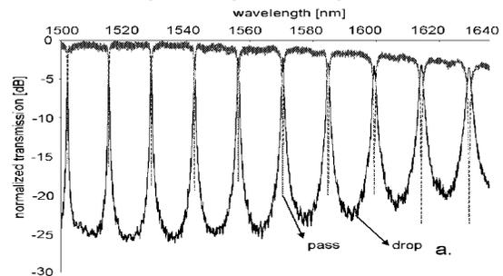
Fig.1 Pass and drop transmission spectra of a racetrack resonator with a bend radius of 5 micron.
