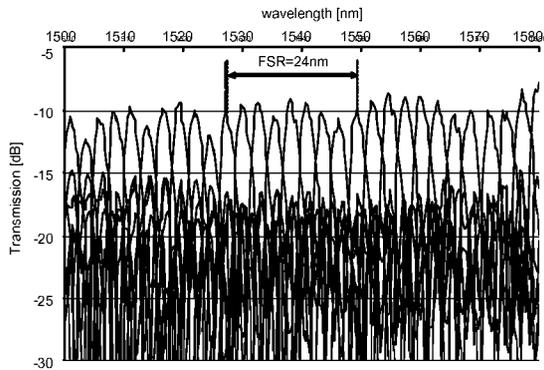
Fig. 2 Microscope image of the 8channel AWG and superimposed plot of the 8 transmission spectra.
