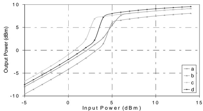
Fig. 2 Calculated static decision characteristics for different coupling factors and drive currents of both SOA and laser diode. (a)  $x=0.5$ ,  $I_{laser}=120\text{mA}$  and  $I_{SOA}=90\text{mA}$ , (b)  $x=0.6$ ,  $I_{laser}=120\text{mA}$  and  $I_{SOA}=90\text{mA}$ , (c)  $x=0.5$ ,  $I_{laser}=120\text{mA}$  and  $I_{SOA}=80\text{mA}$ , (d)  $x=0.5$ ,  $I_{laser}=130\text{mA}$  and  $I_{SOA}=90\text{mA}$ .
