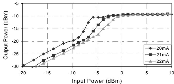
Fig. 4 Tuning of the decision point by adjusting the drive current of the laser diode.
