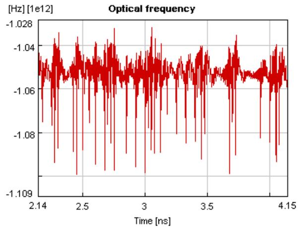
Figure 4 : Variations of the frequency of the laser field for an input signal of 40 Gb/s 1 ps pulses.
