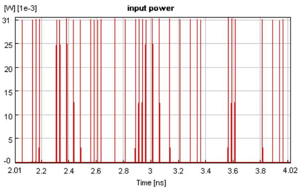
Figure 2 : Input signal of 40 Gb/s 1 ps pulses.
