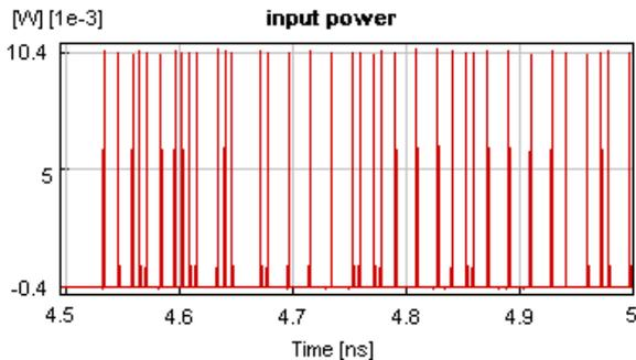
Figure 6 : Input signal for 160 Gb/s.
