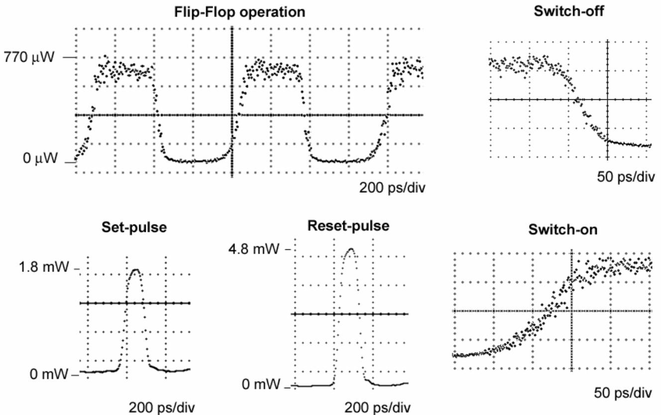
Figure 3: All-optical flip-flop operation using pulses of 100 ps with energy less than 0.5 pJ. Repetition rates up to 1.25 GHz can be obtained and the switch-on time of the laser is only 120 ps.
