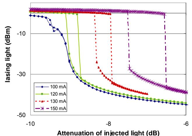
Figure 2: Measured bistability for a  $\lambda/4$ -shifted DFB-laser of 400  $\mu\text{m}$  and different injection currents.
