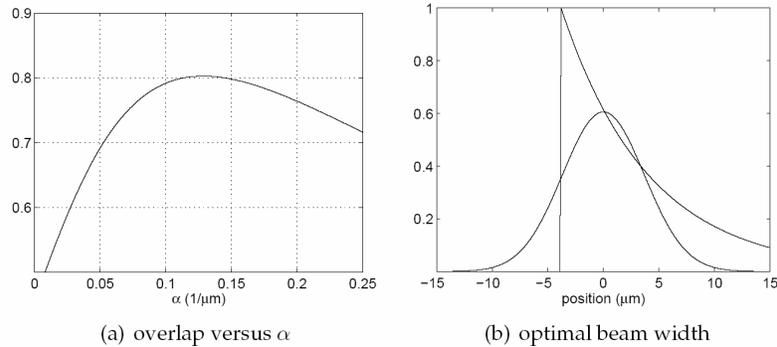
Fig. 3. Overlap of the Gaussian fiber mode and the exponentially decaying diffracted field profile (normalized by the directionality  $D$ )
