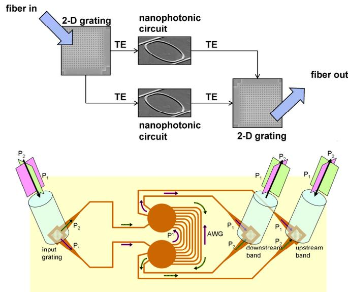
Fig. 7. Polarization diversity based on a two-dimensional diffraction grating: operation principle (top) and practical implementation which avoids the doubling of required integrated components (bottom)
