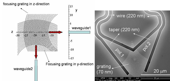
Fig. 9. Design and implementation of a focusing two-dimensional diffraction grating
