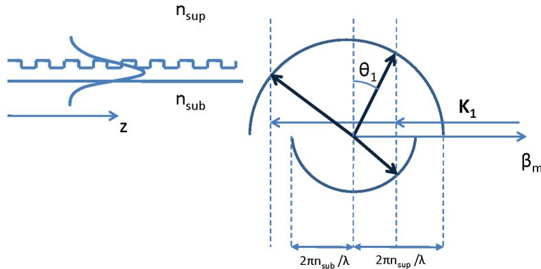
Fig. 1. Bragg vector diagram illustrating the diffraction properties of a periodic structure.
