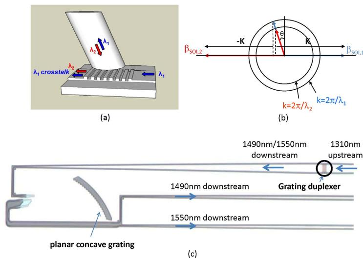
Fig. 5. Grating duplexer structure to couple two wavelength bands to the SOI photonic integrated circuit
