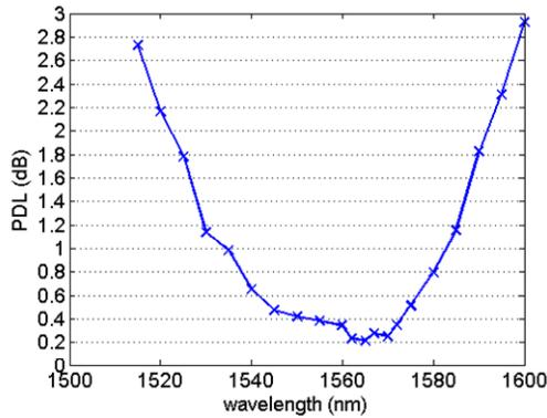
Fig. 8. Wavelength dependence of the polarization dependent loss of two-dimensional grating couplers
