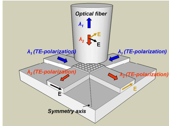
Fig. 10. Two-dimensional grating duplexer layout for polarization independent duplexing of two wavelength bands
