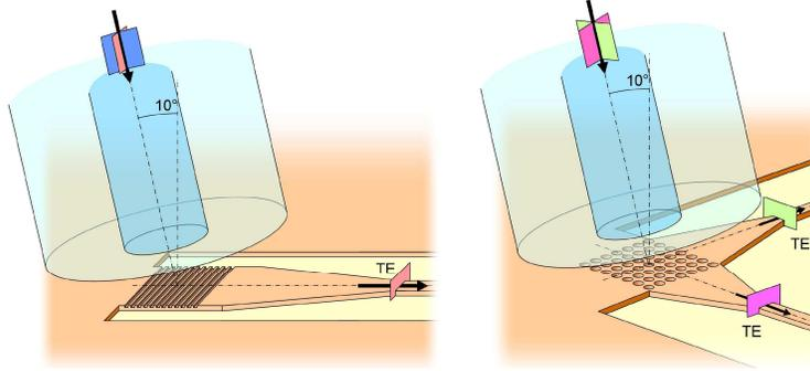
Fig. 6. Operation principle of a two-dimensional diffraction grating.
