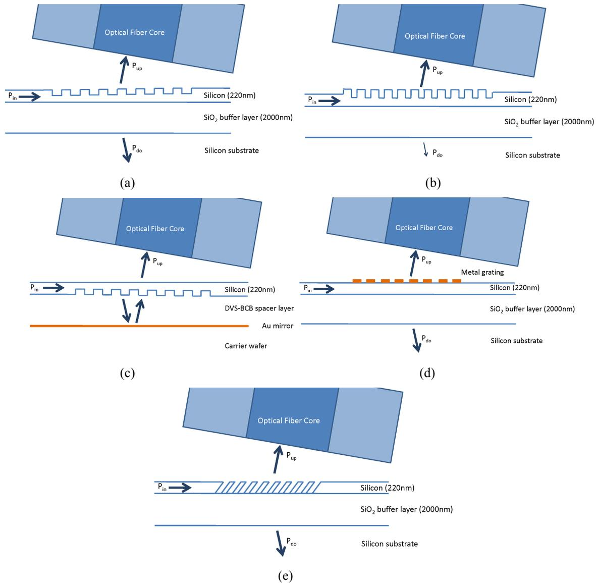
Fig. 2. Studied one-dimensional diffractive grating structures: directly etched gratings (a), raised fiber couplers (b), metallic bottom mirror gratings (c), metallic periodic structures (d) and slanted grating couplers (e).
