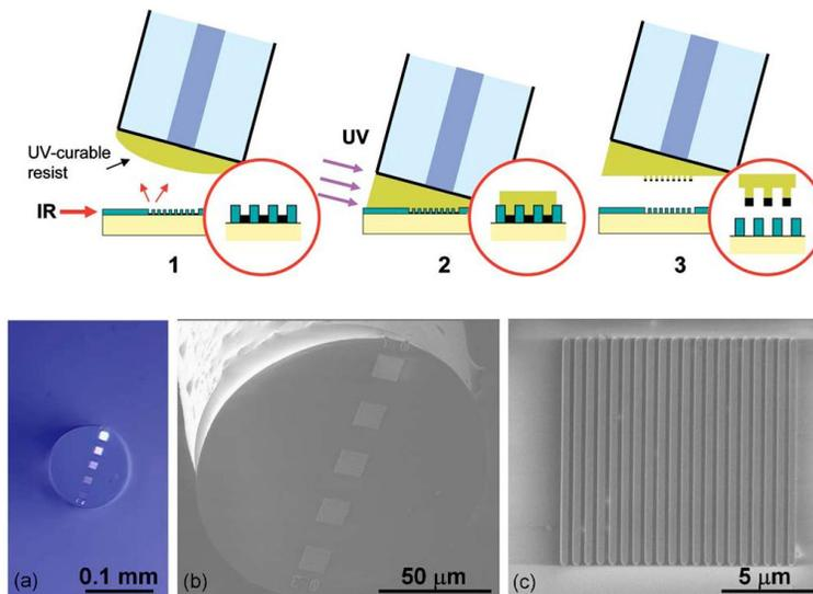
Fig. 11. Fabrication flow (a) and experimental realization (b) of optical fiber probes
