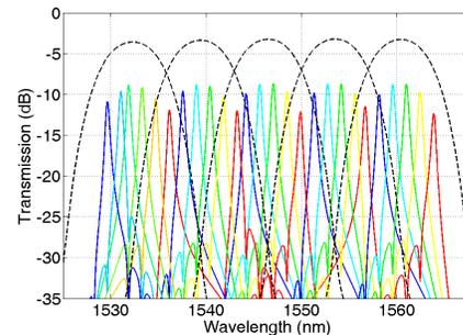
Figure 1. Simulated spectral response of the of the PCG (dashed lines) and the demultiplexer (solid lines).
