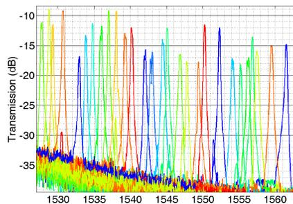
Figure 3. Measured spectral response of the demultiplexer.
