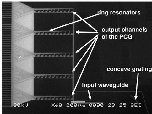
Figure 2. Scanning electron microscope image of the demultiplexer.
