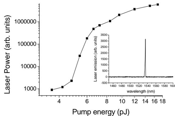
Fig 3. Laserlight-light (log-log) characteristics and spectrum
