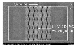
Fig 2. SEM of the 2DPCs aligned to SOI wires
