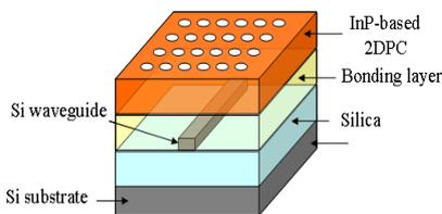
Fig 1. Schematic of the platform
