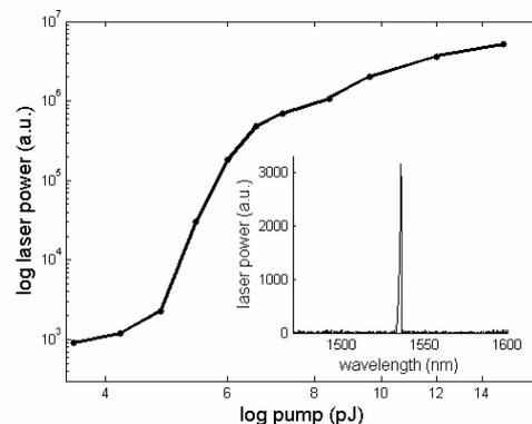
Fig2. Laser light-light (log log) characteristic and spectrum
