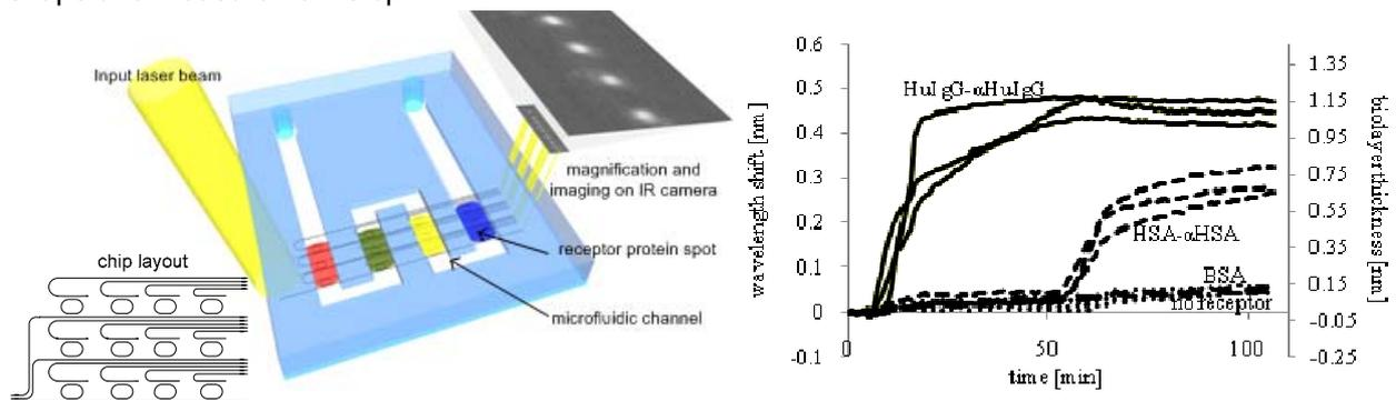
Figure 1. (left) Illustration of the biosensor platform, not to scale. (right) Multiplex biosensing experiment with 3 different molecules spotted on the SOI chip.
