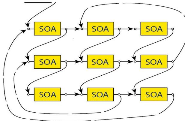
Figure 1. The topology used for the SOA simulations.
