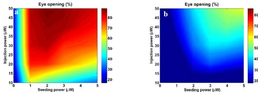
Fig. 3 – Relative eye opening (EO) in % at (a) 10 Gb/s and (b) 20 Gb/s.
