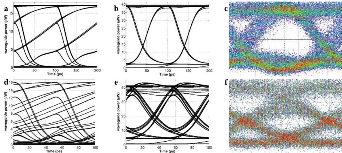
Fig. 4 – Wavelength conversion: Simulation at 10 Gb/s with 50  $\mu$ W injection and (a) without seeding, (b) with 2  $\mu$ W seeding, (c) measurement at 10 Gb/s with seeding. Simulation at 20 Gb/s with 50  $\mu$ W injection and (d) without seeding, (e) with 5  $\mu$ W seeding, (f) measurement at 20 Gb/s with seeding.
