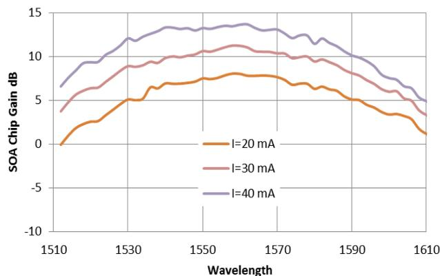
Figure 5. Amplifier gain versus wavelength for different current levels for an amplifier with 400µm length, 2µm width and 100µm taper length
