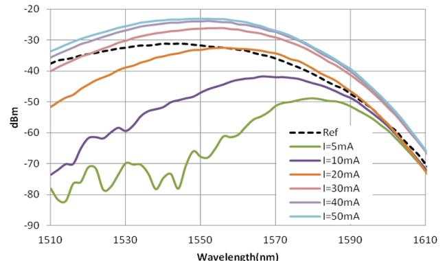
Figure 3. Fiber-to-fiber transmission versus drive current and a reference transmission spectrum.
