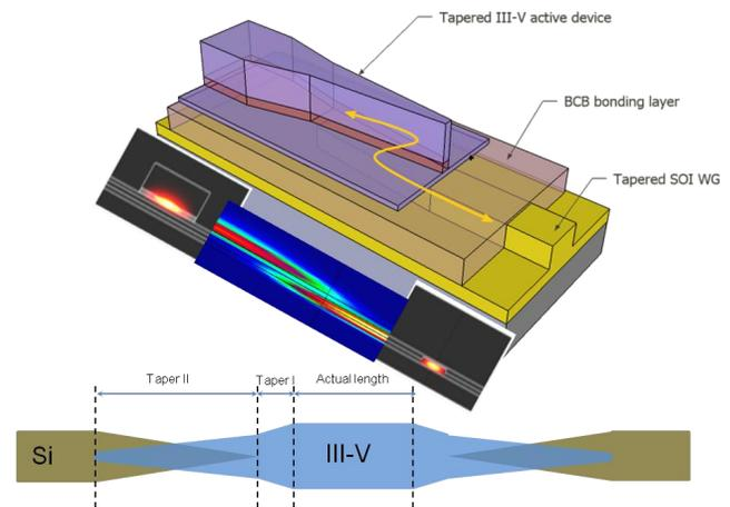
Figure 1. (a) Three-dimensional view of the coupling structure of the hybrid amplifier with representative mode profiles in two cross-sections; (b) the detailed top view of the the hybrid amplifier.
