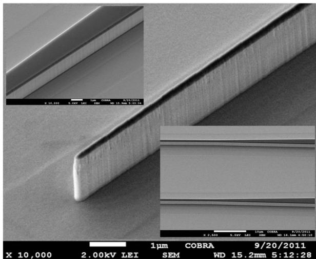
Figure 2. SEM picture of a III-V waveguide and taper tip.
