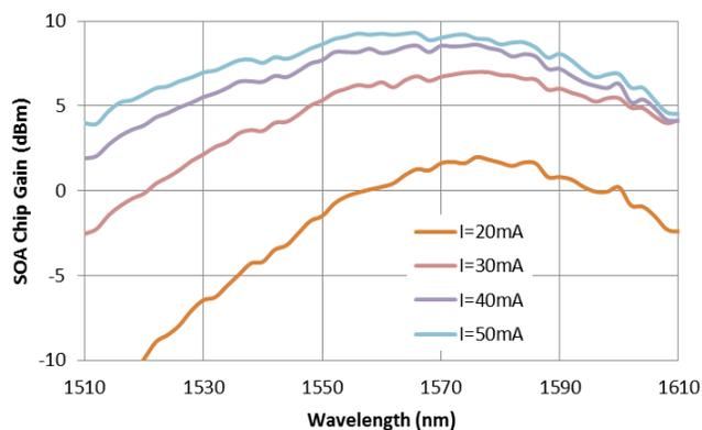
Figure 4. Amplifier gain versus wavelength for different current levels for a 200µm long amplifier with a width of 3µm and 100µm taper length.
