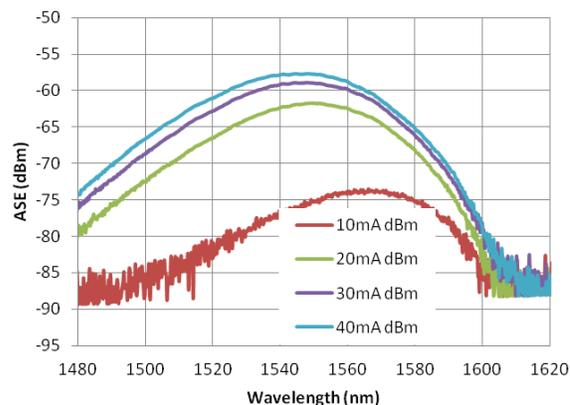
Figure 6. ASE spectra of the amplifier for different applied currents (a) amplifier with 200µm length, 3µm width and 100µm taper length (b) amplifier with 400µm length, 2µm width and 100µm taper length
