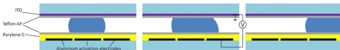
**Fig. 1** The cross section of an electrowetting-on-dielectric (EWOD) lab-on-a-chip and the electrowetting principle. When a voltage is applied to an actuation electrode, the droplet is attracted toward this
