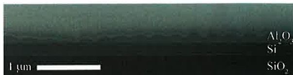
Fig. 4. Cross-section of part of a holographic grating, fabricated by FIB etching.
