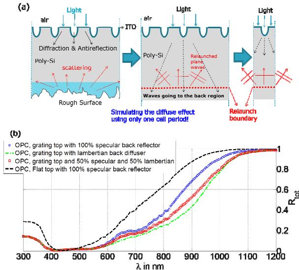
Fig. 2 (a) Modelling schematic of the OPC calculations. (b) Example reflectance of combined structure as compared to an all flat structure assuming poly-Si thickness  $d = 2.5 \mu\text{m}$ .
