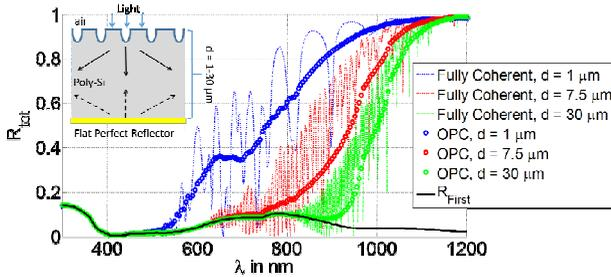
Fig. 1 Reflectance curves under fully coherent and one pass coherent conditions for top grating-flat bottom solar cell structures with different Si thicknesses.
