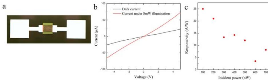
Figure 3. (a) microscope picture of a  $S^{2-}$  -terminated PbS colloidal QD photodetector. (b) Current-voltage characteristics of processed  $S^{2-}$  -terminated PbS colloidal QD photoconductors. (c) Responsivity dependence as a function of optical power at  $1.55 \mu m$  and a bias voltage of 10 V for an  $S^{2-}$  -terminated PbS colloidal QD photodetector.
