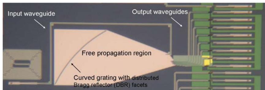
Figure 4. microscope picture of a  $\text{OH}^-$ -terminated PbS colloidal QD photodetector array integrated on a planar concave grating spectrometer.
