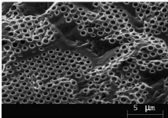
Fig. 2. SEM picture of a nanopatterned PolySi layer
