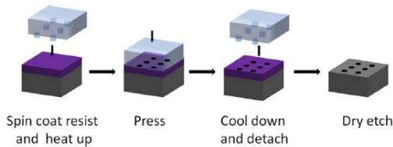
Fig. 1. Schematic representation of the soft thermal-nanoimprint lithography process flow [6]
