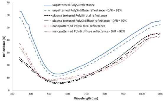
Fig. 5. Total and diffuse reflectance of an unpatterned, plasma textured and nanopatterned PolySi layer
