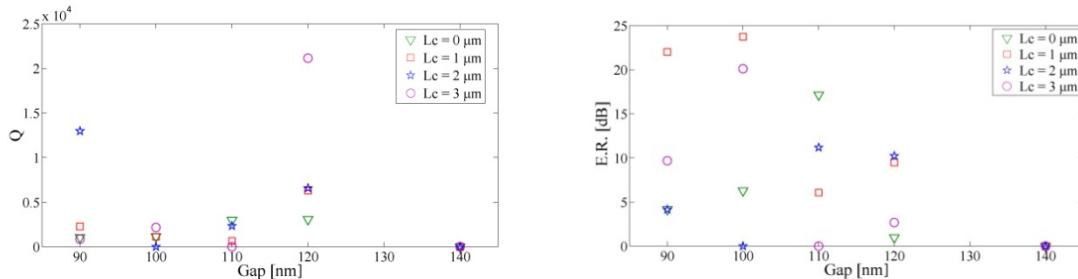
Figure 2. Measured Q (a) and ER(b) of a TE mode for a ring with water cladding and a width of 550 nm in function of the gap of the coupling section, for various coupling lengths.
