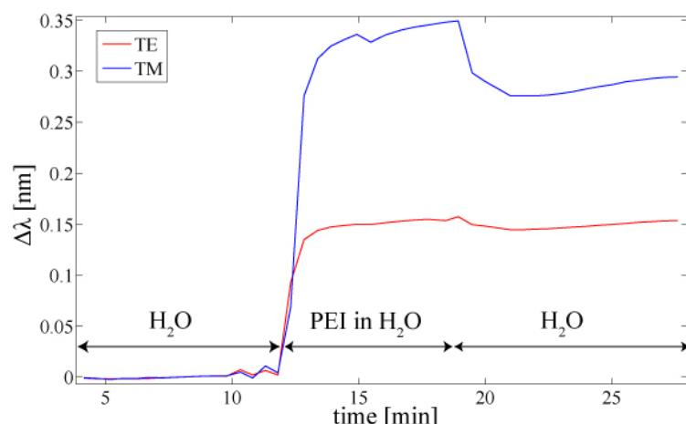
Figure 3. Shift of the resonant wavelength for a TE mode at  $\lambda=1542 \text{ nm}$  and a TM mode at  $\lambda=1536 \text{ nm}$ , during the adsorption of a 2mg/ml solution of PEI in water on the silicon surface of the microring.
