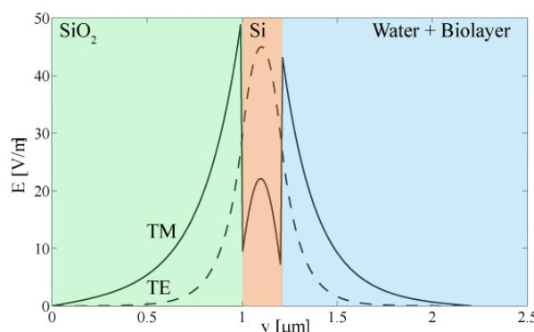
Figure 1. Electric field profile of quasi-TE and quasi-TM mode in the horizontal centre of the 2D waveguide cross section, as a function of the vertical coordinate. For both polarisations, only the dominant electric field component in the 2D cross section is shown.
