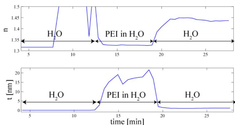
Figure 4. Refractive index and thickness profile of the adsorption of PEI on the silicon surface of the microring.
