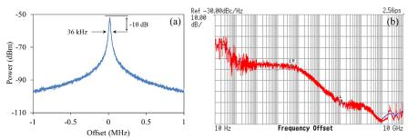
Fig. 5. (a) Zoom of the main RF tone, indicating a 36 kHz –10dB bandwidth; (b) phase noise spectrum of the main RF tone at 4.69 GHz. The timing jitter is 2.56 ps when integrated from 50 kHz to 10 MHz. Resolution bandwidth, video bandwidth and sweep time used to obtain the RF spectra in (a) were 2 kHz, 20 Hz, and 40 s respectively.
