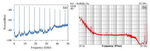
Fig. 11. (a) Wide band electrical spectrum under hybrid mode-locking; (b) phase noise spectrum of the main RF tone at 4.65 GHz under hybrid mode-locking. Resolution bandwidth, video bandwidth and sweep time used to obtain the RF spectra in (a) were 500 kHz, 50 kHz, and 1.5 s respectively.
