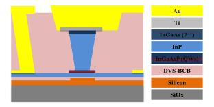
Fig. 1. Cross-section of the III-V-on-silicon waveguide structure.
