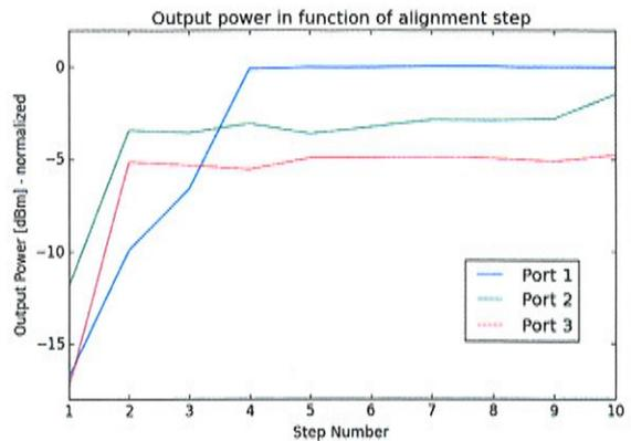
Fig. 4. Evolution of the output power at the circuit along the optimization process, when the fiber is positioned at different output.
