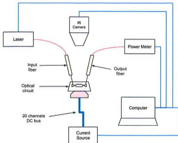
Fig. 3. Measurement setup. Fibers are used for optical input and output, while an IR camera is used to capture the in-circuit monitors. Heaters are driven through a 20-probe array.
