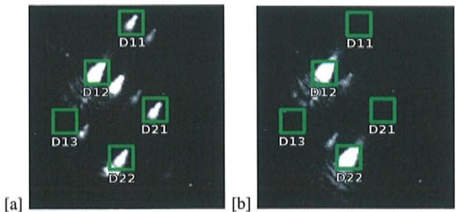
Fig. 5. Intermediate monitors ass seen from the IR camera. The grating couplers in the image that are not labeled as detectors are reflection monitors and were not used in the experiment.
