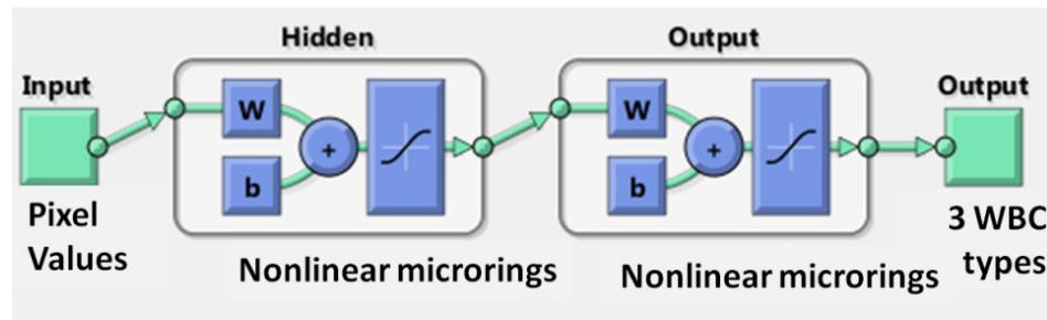
*Figure 2. Schematic of the optical neural network [7] upon which the pattern detection depends. The pixel values from the input and can be realized by grating arrays. The nonlinear transmission function of each neuron in the hidden and output layer is realized by thermal microrings. Three different WBCs are distinguished at the output side.*
