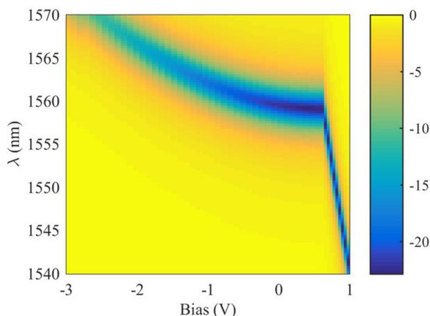
FIG. 4. The simulated exciton absorption spectra (dB) for the 80 μm long EAM with different bias voltages. The strongest absorption is more than 20 dB.
