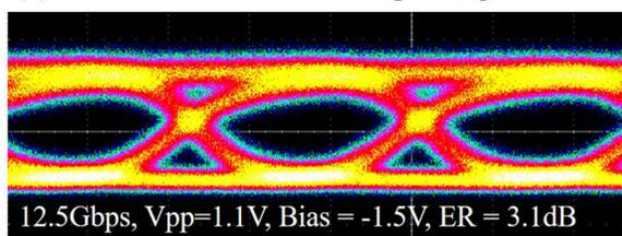
FIG. 6. Measured  $2^{31}-1$  PRBS NRZ eye diagrams at  $1.55\ \mu\text{m}$  (a) 1.25 Gbps at forward bias 0.6 V. (b) 12.5 Gbps at reverse bias  $-1.5\ \text{V}$ .
