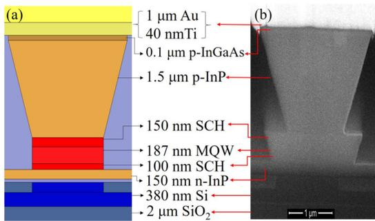
FIG. 1. (a) Cross-sectional view of the EAM bonded on SOI. (b) SEM image of the cross-section of the fabricated III-V/Si hybrid waveguide.
