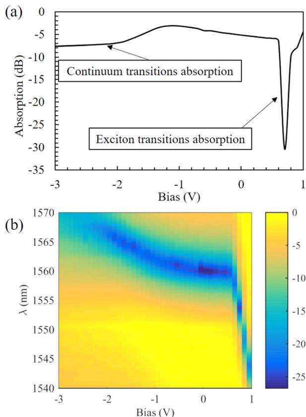
FIG. 5. (a) The bias dependent absorption for the  $80\ \mu\text{m}$  long EAM at  $1.55\ \mu\text{m}$ . (b) The exciton absorption spectra (dB) for different bias voltages. The strongest absorption is more than 20 dB.
