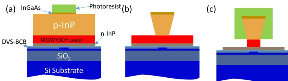
FIG. 2. The fabrication process of the III-V waveguide.
