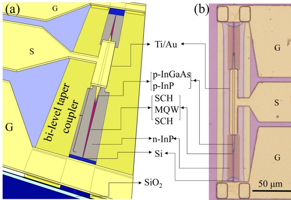
FIG. 3. (a) Three-dimensional sketch of the EAM bonded on SOI. (b) Top microscope image of the III-V/Si hybrid integrated EAM.
