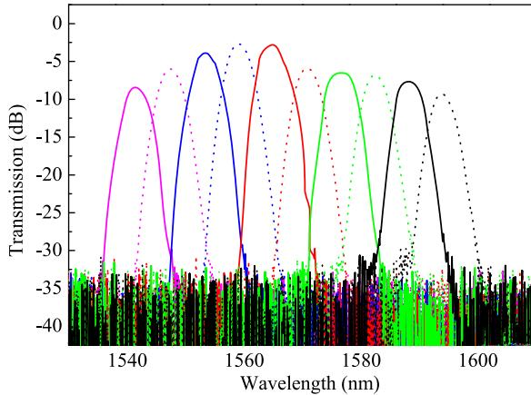
Fig. 5. Measured transmission of a 10 channel PCG fabricated on LPCVD SiN with  $0.3 \mu\text{m}$  guiding and  $3.3 \mu\text{m}$  BOX layers respectively [43].
