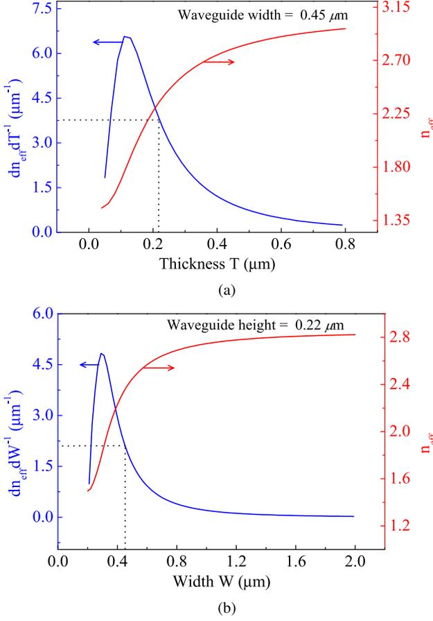
Fig. 3. Effective index (red) and its variation (blue) for the fundamental TE mode of silica cladded SOI strip waveguide (a) with thickness  $T$  for  $0.45 \mu\text{m}$  wide waveguide and (b) with width  $W$  for  $0.22 \mu\text{m}$  thick silicon guiding layer.
