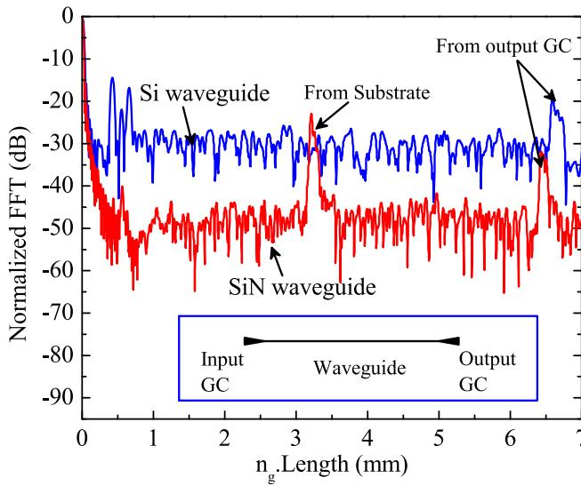
Fig. 2. Spurious reflections in SOI (blue line) and SiN (red line) single mode oxide cladded strip waveguides for TE polarized light. The schematic of the test waveguides for spurious reflections. GC stands for Grating Coupler and  $n_g$  stands for the group index of the waveguide.
