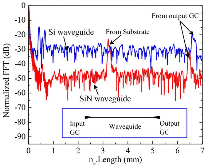
Fig. 2. Spurious reflections in SOI (blue line) and SiN (red line) single mode oxide cladded strip waveguides for TE polarized light. The inset shows the schematic of the test waveguides for spurious reflections. GC stands for the Grating Coupler and  $n_g$  stands for the group index of the waveguide.
