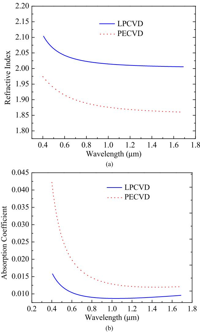
Fig. 1. Refractive index (top) [43] and absorption coefficient (bottom) of typical LPCVD (blue) and PECVD (dotted red) SiN for the visible and IR wavelength regime.
