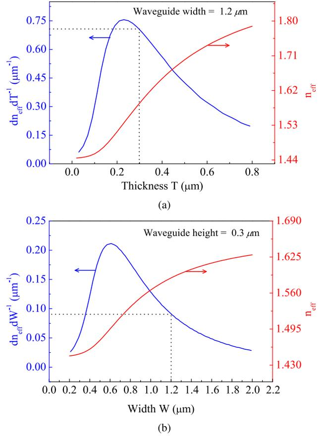
Fig. 4. Effective index (red) and its variation (blue) for the fundamental TE mode of silica cladded SiN strip waveguide (a) with thickness  $T$  for  $1.2 \mu\text{m}$  wide waveguide and (b) with width  $W$  for  $0.3 \mu\text{m}$  thick SiN guiding layer.
