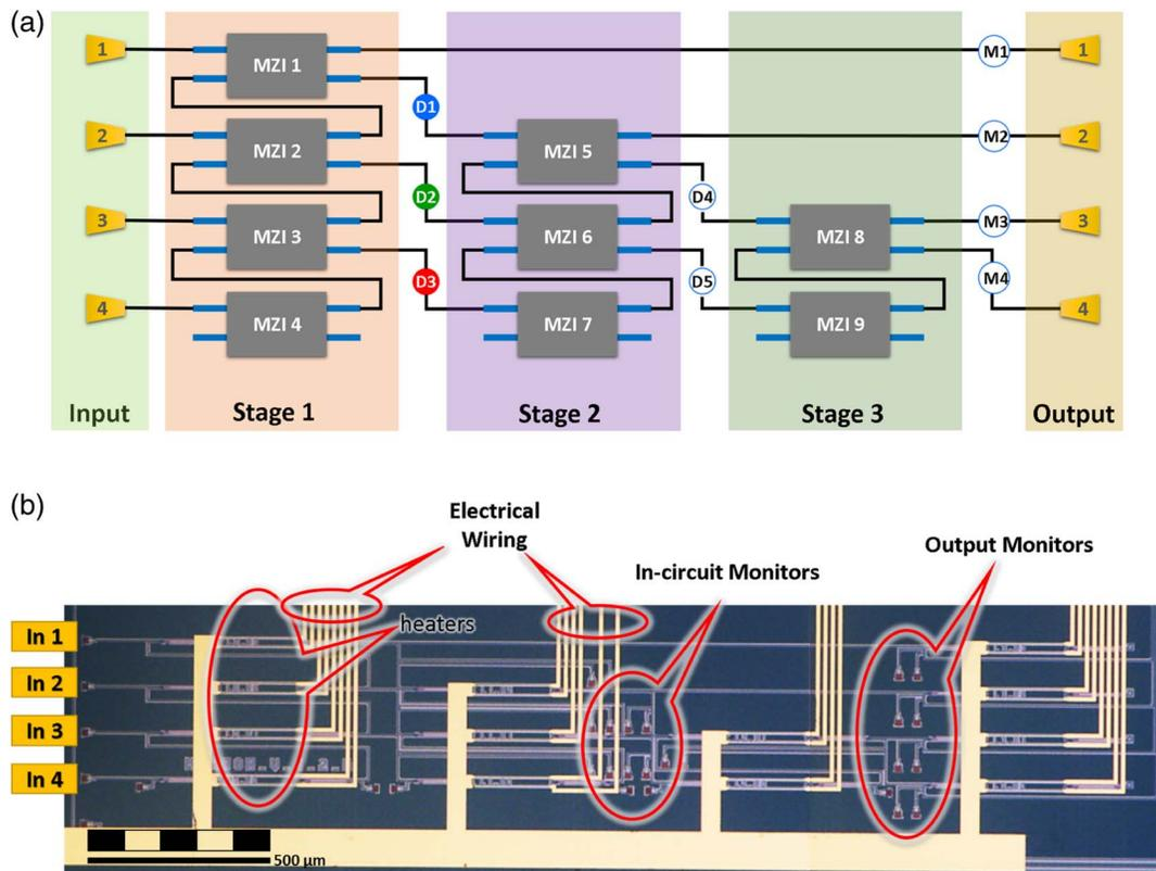
**Fig. 2.** (a) Schematic of the integrated implementation of the circuit using MZIs. The optical input and the output are done using grating couplers. Detectors D1 to D5 are implemented using optical taps connected to a grating coupler, for monitoring using an IR camera. The same approach was used with output monitors M1 to M4, which are used to monitor the optical power at the output of the circuit. (b) Microscope image of the fabricated device.
