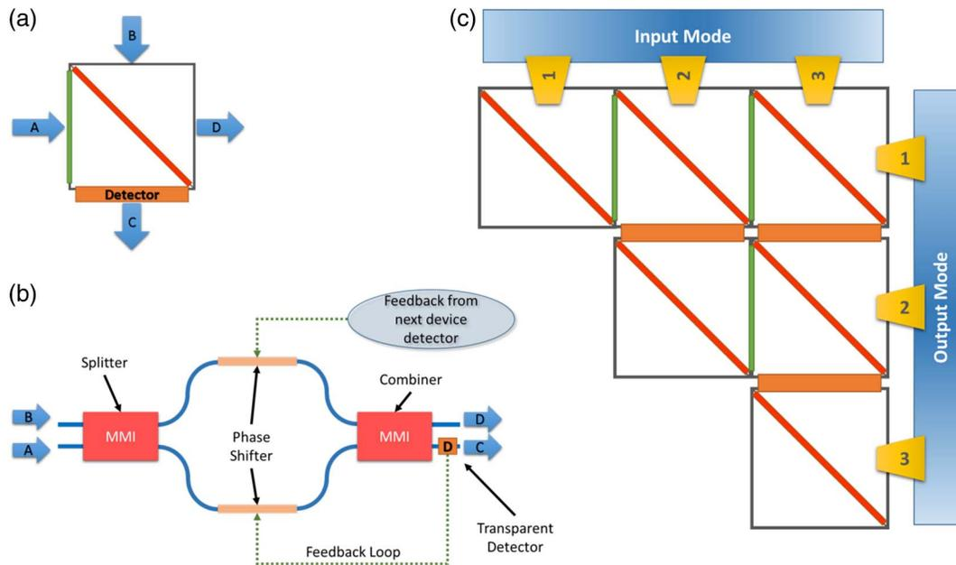
**Fig. 1.** (a) Representation of an individual cell of the circuit with two inputs (A and B) and two outputs (C and D). The green rectangle is a tunable phase shifter and the red rectangle is a semi-transparent mirror with tunable reflectivity. The orange rectangle is a “transparent” photodetector. (b) Mach-Zehnder implementation of the unit cell. (c) A discrete representation of the proposed device from cascaded discrete unit cells.
