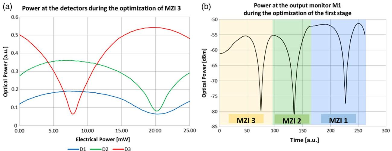
**Fig. 4.** (a) Optical power at the detectors D1, D2, and D3 during the optimization of MZI 3. (b) Evolution of the output power at Out 1 during the optimization of the first stage. The optical power was recorded from the monitor M1, which taps the light from Out 1.
