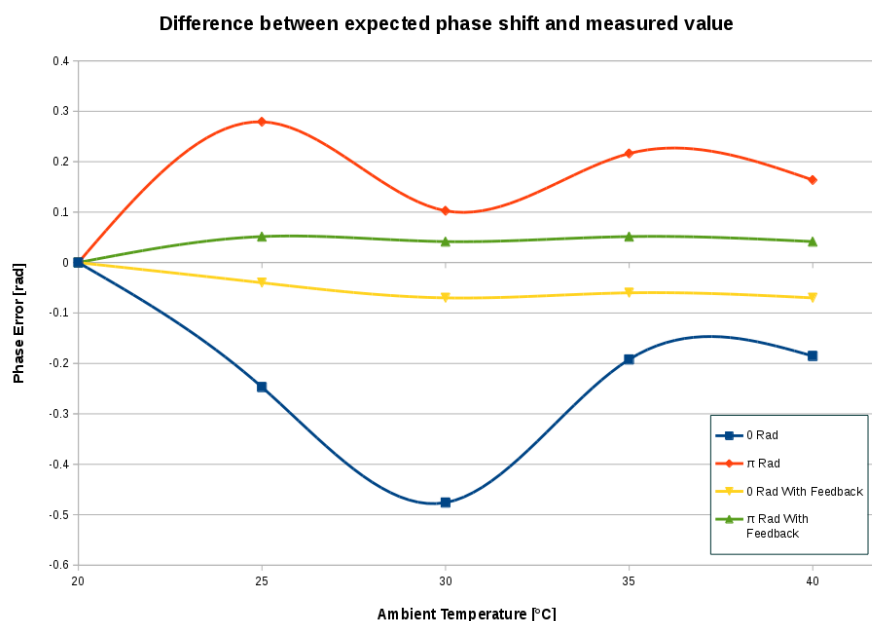
Figure 4: Phase error induced by the change in the ambient temperature. The heater was tuned to delivery a specific phase shift (either 0 Rad or \pi Rad) at 20°C and the phase shift was measured for different ambient temperatures with and without the feedback system actuating.
