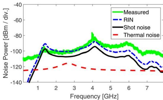
**FIGURE 6** Noise contributions (Resolution bandwidth = 10 kHz). [Color figure can be viewed at [wileyonlinelibrary.com](http://wileyonlinelibrary.com)]
