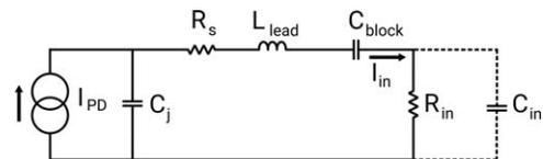
**FIGURE 3** Input circuitry TIA: Series inductive peaking
