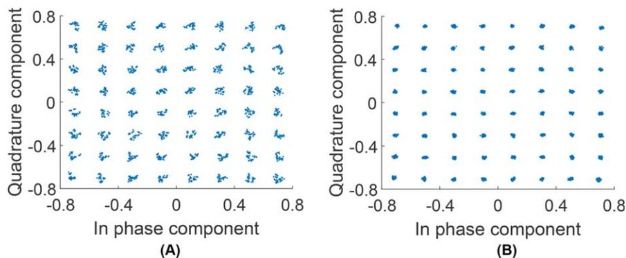
**FIGURE 7** Constellation diagram: 64-QAM, 150 MBaud, 4 GHz carrier, root raised cosine filter (roll-off = 0.5) at receiver and transmitter (A) No equalization (B) 3 taps equalization. [Color figure can be viewed at [wileyonlinelibrary.com](http://wileyonlinelibrary.com)]
