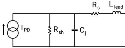
**FIGURE 1** Equivalent network of a PIN PD
