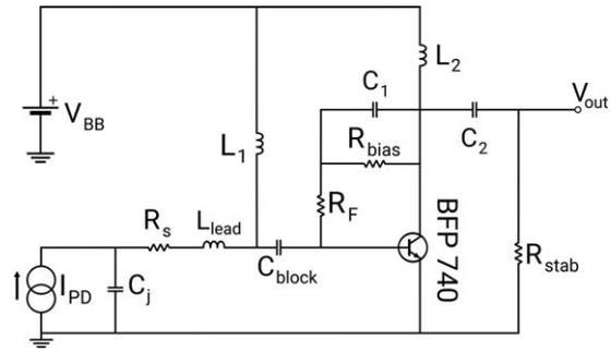
FIGURE 4 TIA design using series inductive peaking
