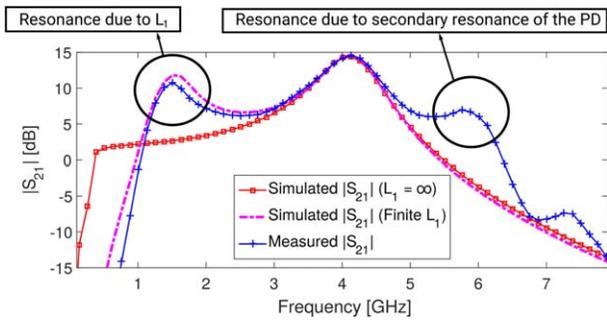
**FIGURE 5** Measured  $S_{21}$  compared to simulated  $S_{21}$ . [Color figure can be viewed at [wileyonlinelibrary.com](http://wileyonlinelibrary.com)]
