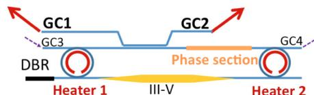
Fig. 1. Schematic of the unidirectional, widely-tunable and narrow-linewidth III-V-on-silicon laser.
