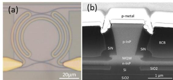
Fig. 4. (a) Microscope image of the ring resonator with a TiAu micro-heater to tune the emission wavelength. (b) SEM cross-section image of the III-V-on-silicon waveguide structure in the middle of the taper section showing good alignment between the III-V waveguide and the underlying silicon waveguide.
