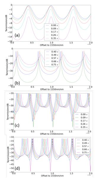
Fig. 2. Figures showing the simulated spectra of the embedded FP cavity (a) and (c), as well as the complete device (b) and (d).
